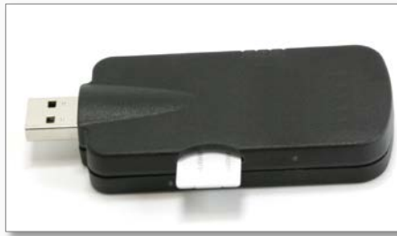
Figure 5.b: Push it forward into the SIM-holder until it stops.
