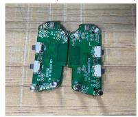
2. The left (L) and right (R) frames of the main board are mirror images, and the front and back sides are distinguished by silk screen L/R (see Figure:)
