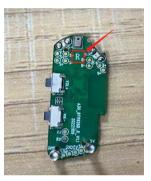
3. The left and right motherboard is a common schematic, a common software, hardware to distinguish the left and right ear function; The ADC2/PA7 is grounded for the left ear and suspended for the right ear (see figure:)
