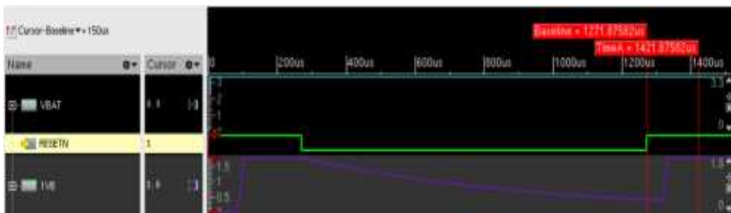
Figure 8. Typical Timing Diagram for Reset Sequence
