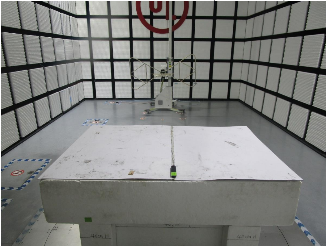
RADIATED RF MEASUREMENT SETUP (Below 30 MHz)
