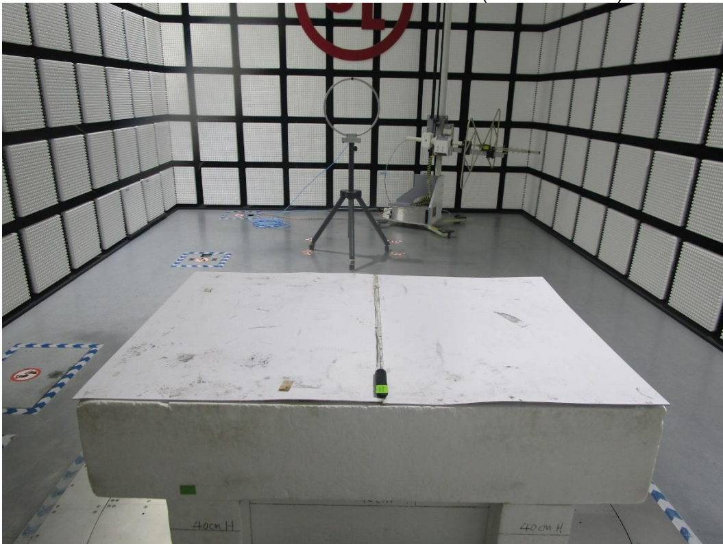
RADIATED RF MEASUREMENT SETUP (Below 30 MHz)
