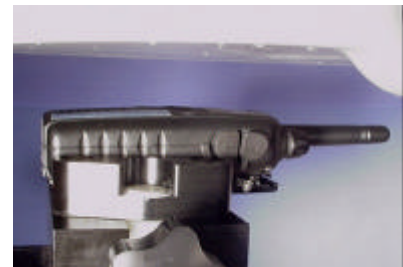
Face-held SAR Test Setup 2.5cm Separation Distance
