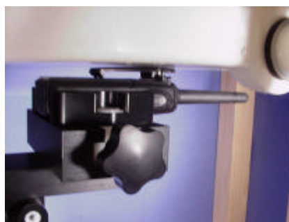
Body-worn SAR Test Setup with 1.0cm Belt-Clip
