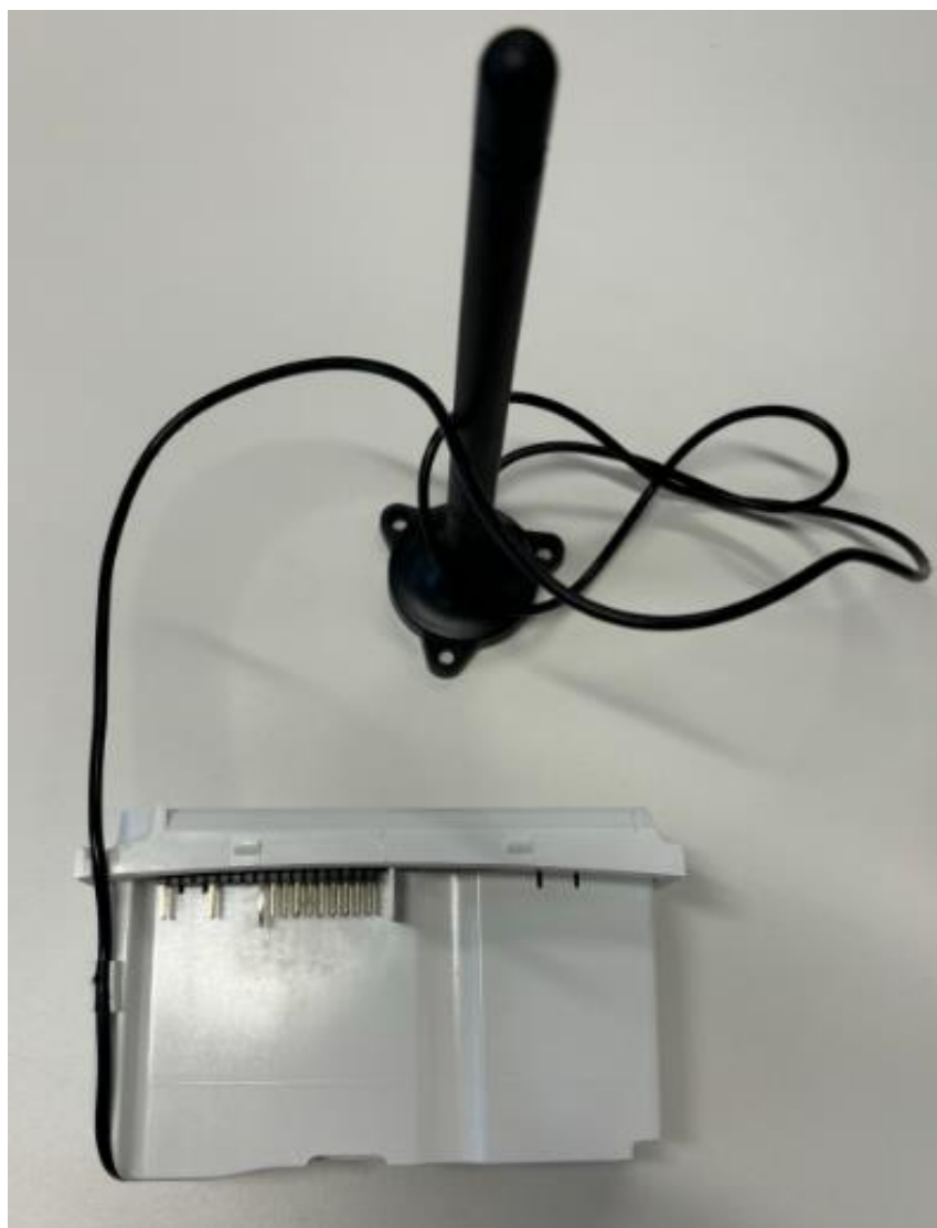
Figure 19 - GLOBYTGNG3 communication module with external antenna top side
