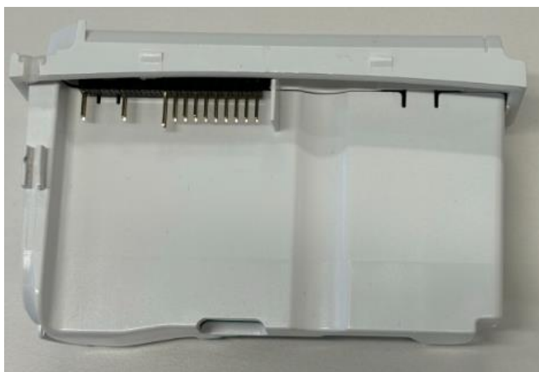
Figure 15 - GLOBYTNG3 communication module with internal antenna bottom side
