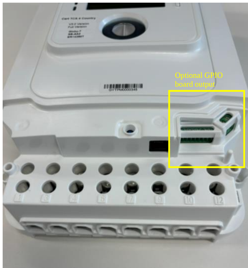
Figure 9 - GLOBYTNG3 bottom side open full version
