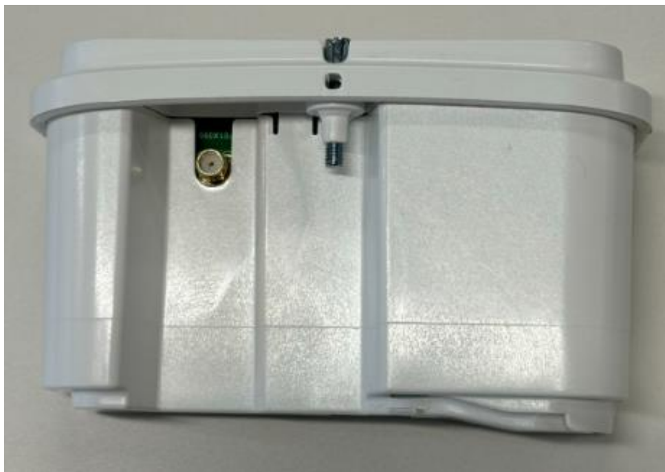
Figure 14 - GLOBYTNG3 communication module with internal antenna top side
