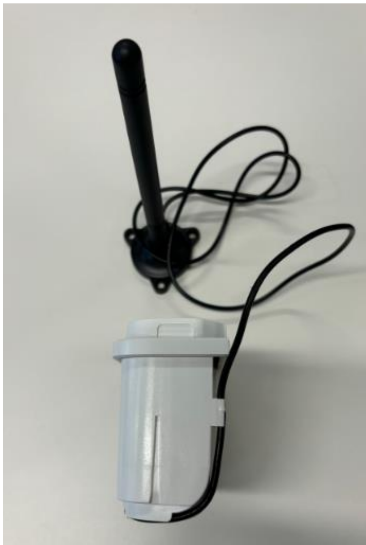
Figure 20 - GLOBYTGNG3 communication module with external antenna right side
