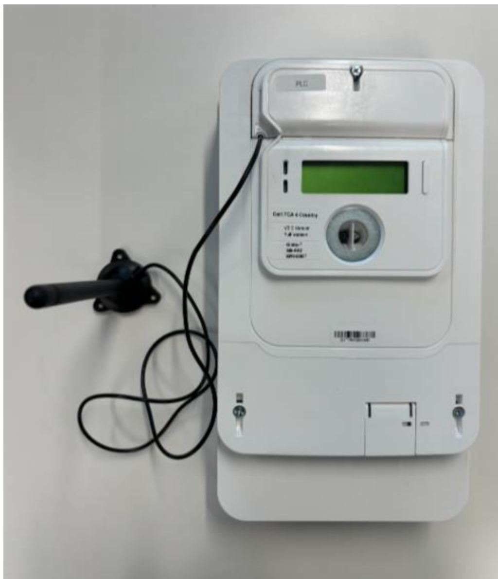
Figure 3-GLOBYTGNG3 front side with external antenna full version
