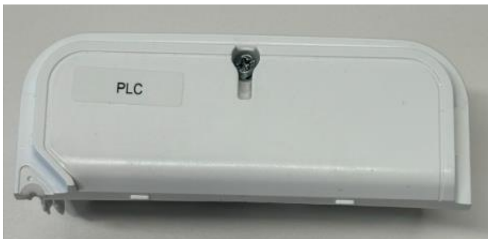
Figure 12 - GLOBYTGNG3 communication module with internal antenna front side
