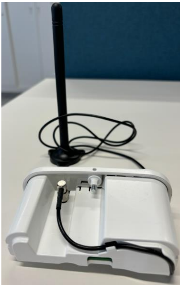
Figure 18 - GLOBYTGNG3 communication module with external antenna
