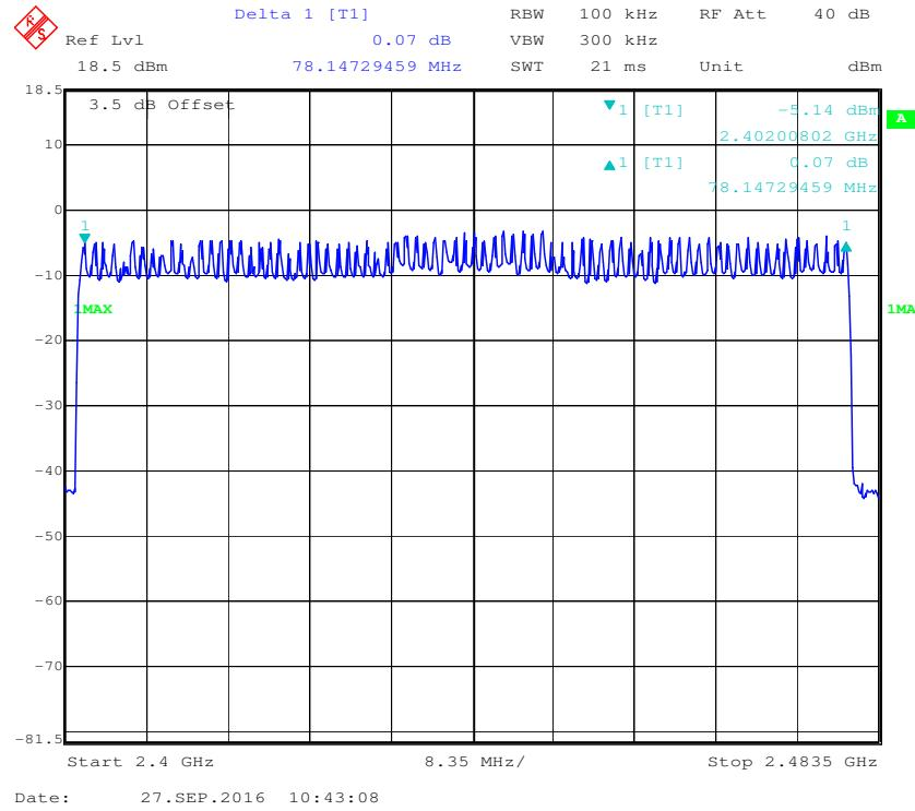
**EDR (8DPSK): Number of Hopping Channels**
