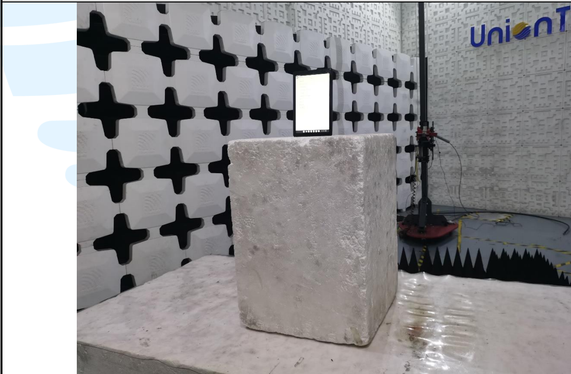
Radiated emission Test Setup (Above 1 GHz)
