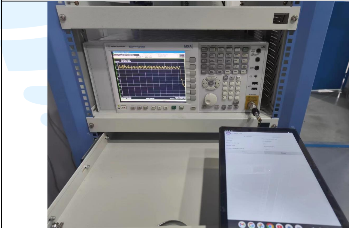
RF Conducted Test Setup
