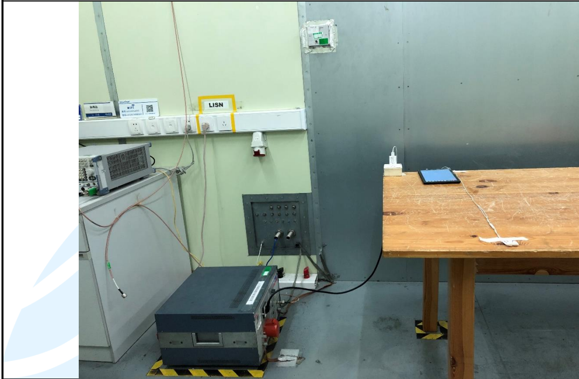
Conducted Emission Test Setup
