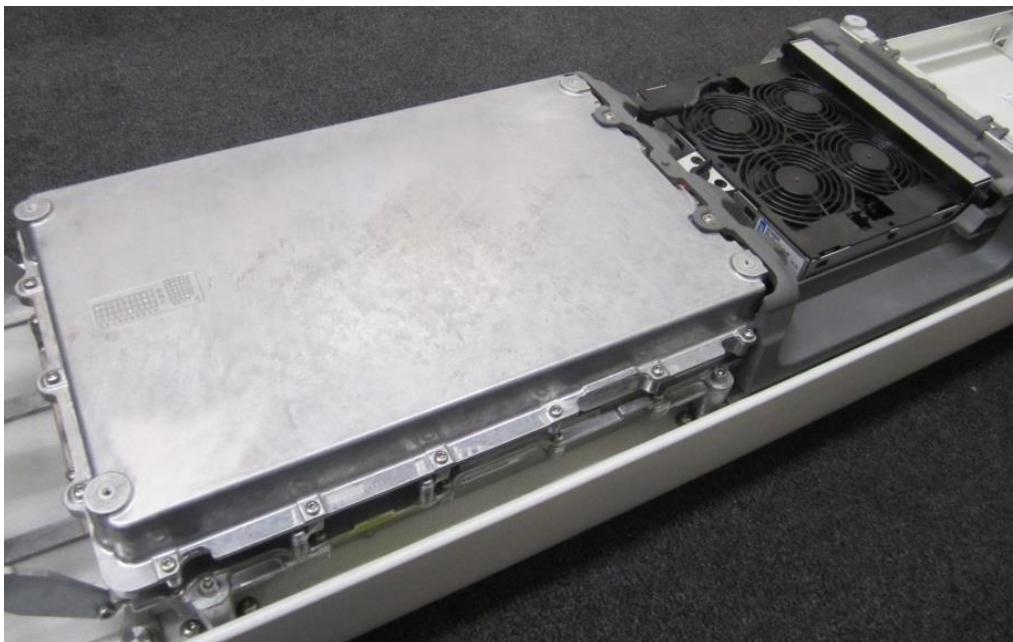
Figure 10.1-3: RRUS 32A B66A with Fan Tray
