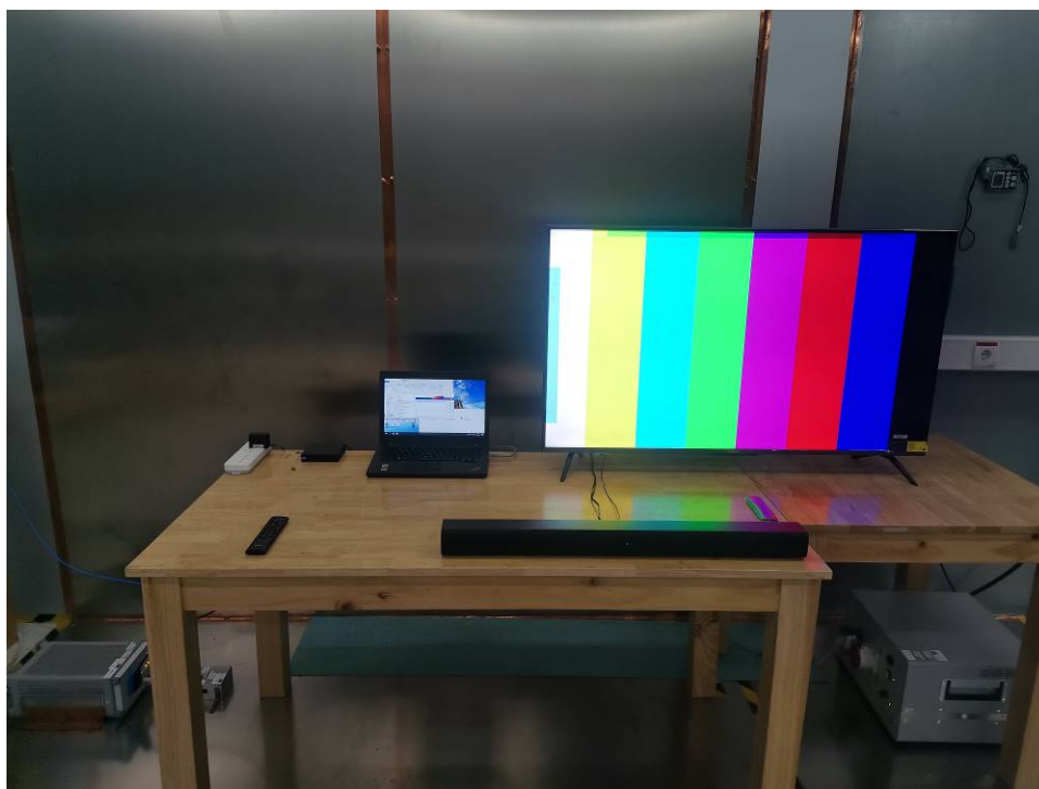
Photograph 3: Set-up for Conducted Emission on AC Mains
