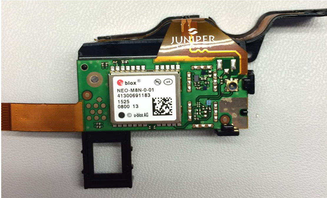
MS2 GNSS flex (front)
