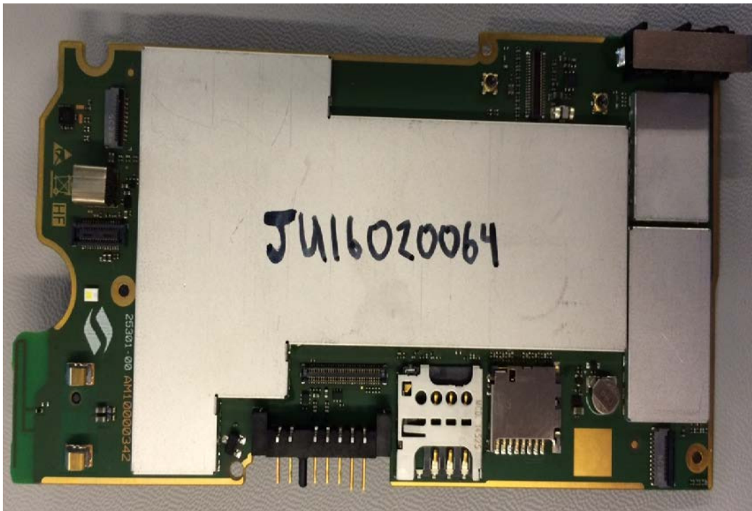
MS2 main PCBA (front) with shields
