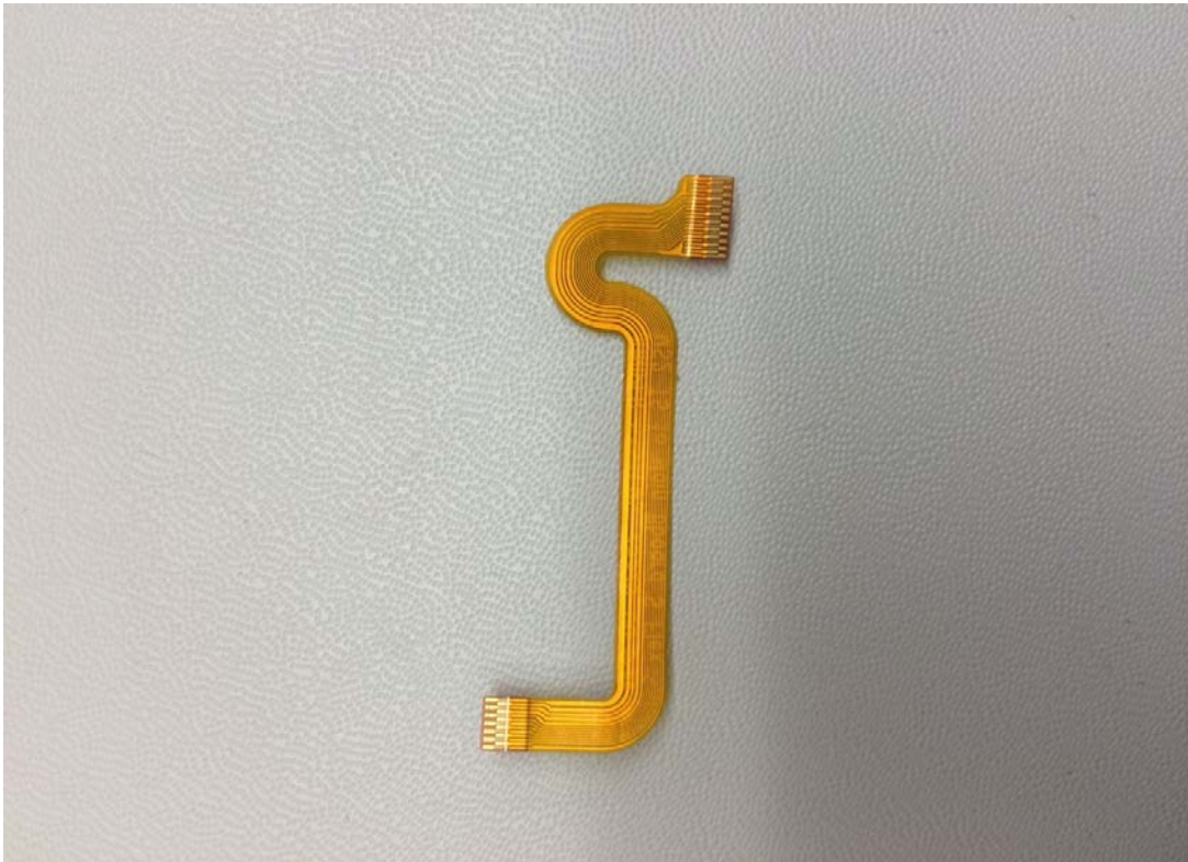
MS2 "S" connector flex (back)
