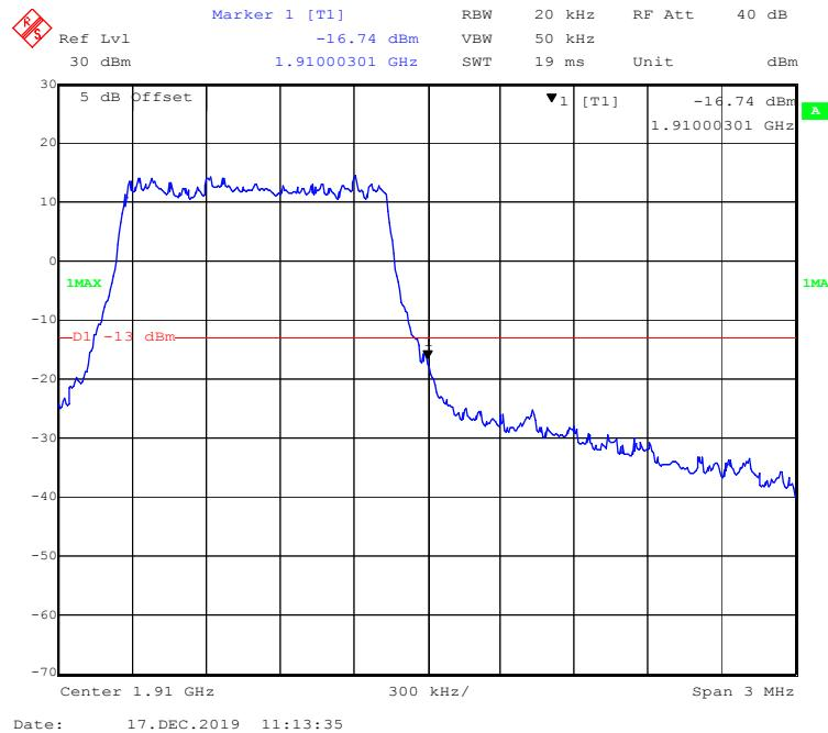
**16-QAM (3 MHz, FULL RB) - Left Band Edge**
