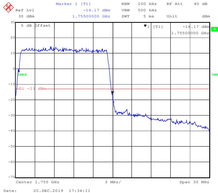
**16-QAM (20 MHz, FULL RB) - Left Band Edge**
