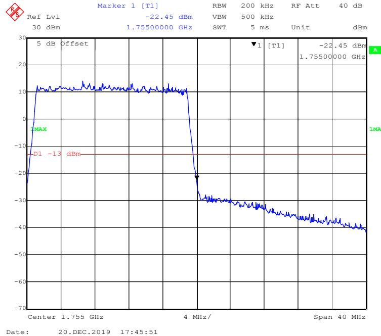
**LTE Band 5:****QPSK (1.4 MHz, FULL RB) - Left Band Edge**
