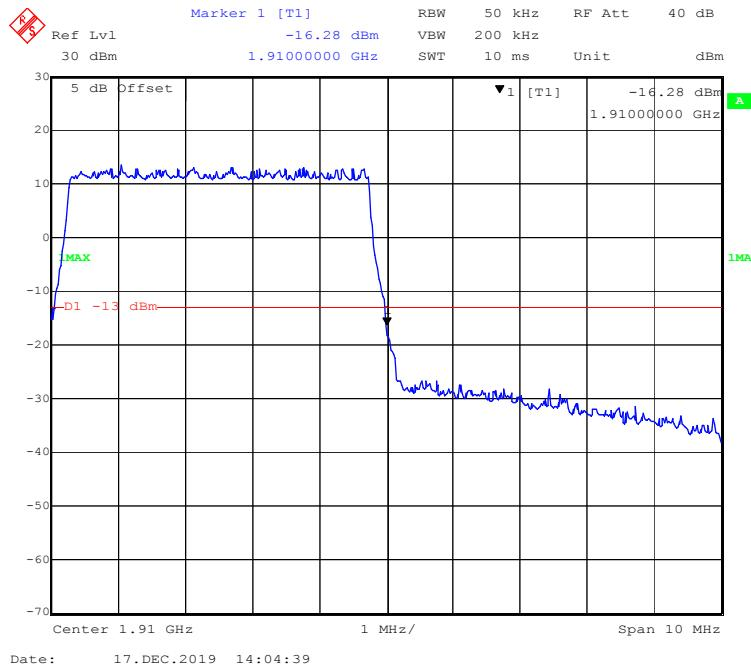
**16-QAM (10 MHz, FULL RB) - Left Band Edge**
