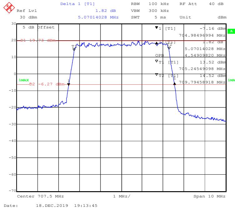
**16-QAM (10 MHz) - 99% Occupied & 26 dB Emissions Bandwidth, Middle channel**
