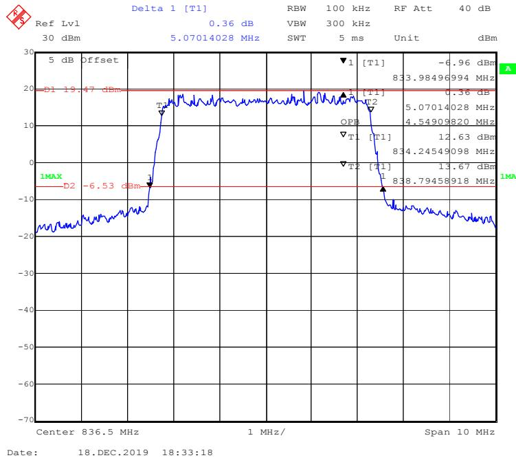
**16-QAM (10 MHz) - 99% Occupied & 26 dB Emissions Bandwidth, Middle channel**
