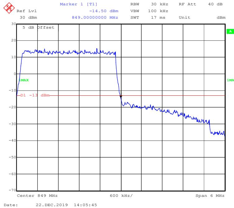
**QPSK (5 MHz, FULL RB) - Left Band Edge**
