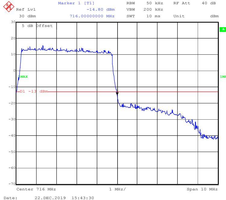
**QPSK (10 MHz, FULL RB) - Left Band Edge**
