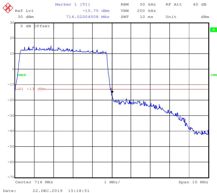
**16-QAM (10 MHz, FULL RB) - Left Band Edge**
