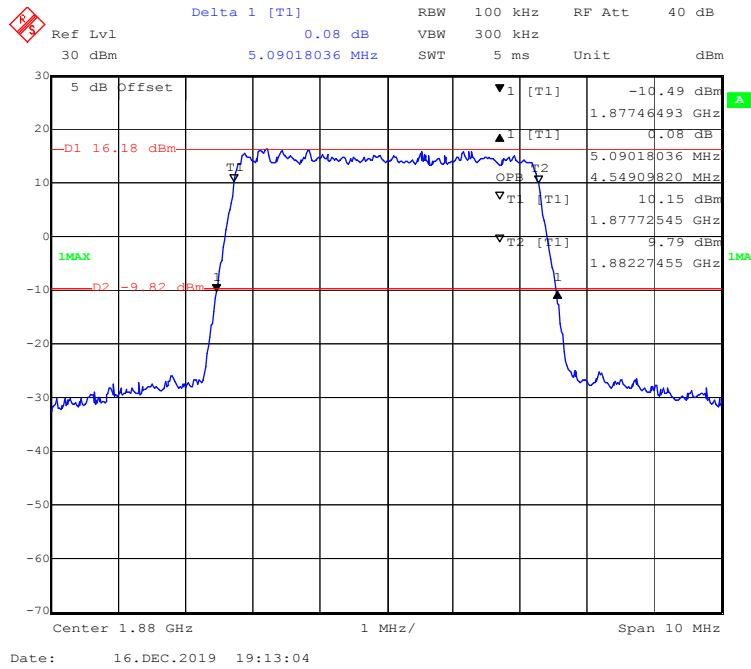
**16-QAM (10 MHz) - 99% Occupied & 26 dB Emissions Bandwidth, Middle channel**
