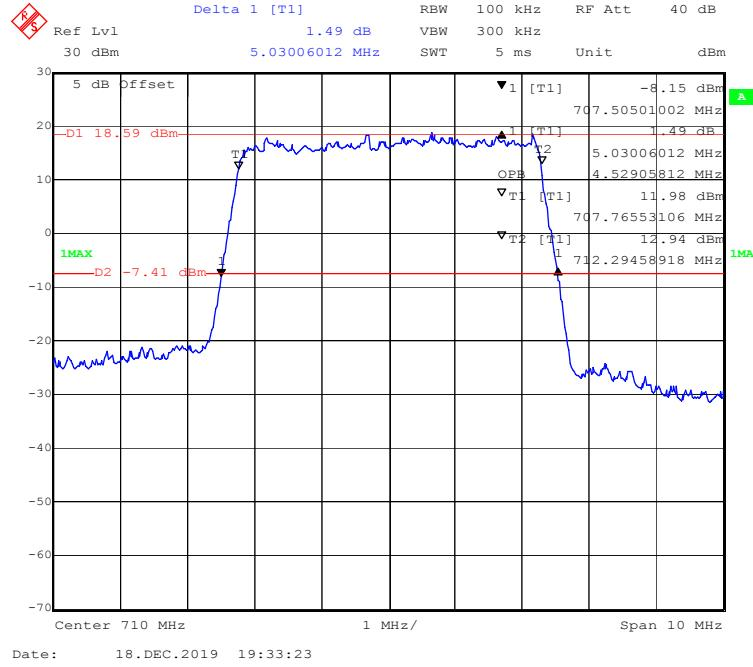
**16-QAM (10 MHz) - 99% Occupied & 26 dB Emissions Bandwidth, Middle channel**
