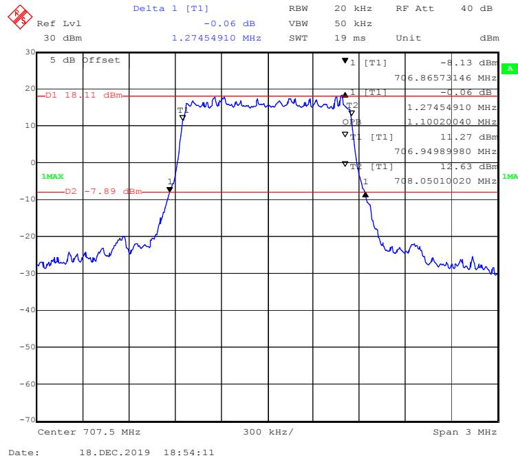
**16-QAM (3 MHz) - 99% Occupied & 26 dB Emissions Bandwidth, Middle channel**
