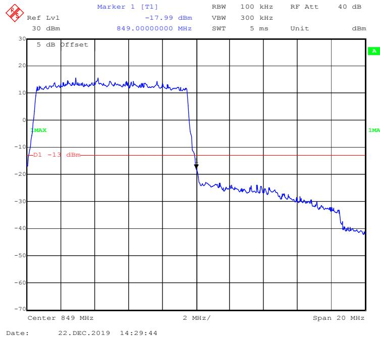
**LTE Band 12:****QPSK (1.4 MHz, FULL RB) - Left Band Edge**
