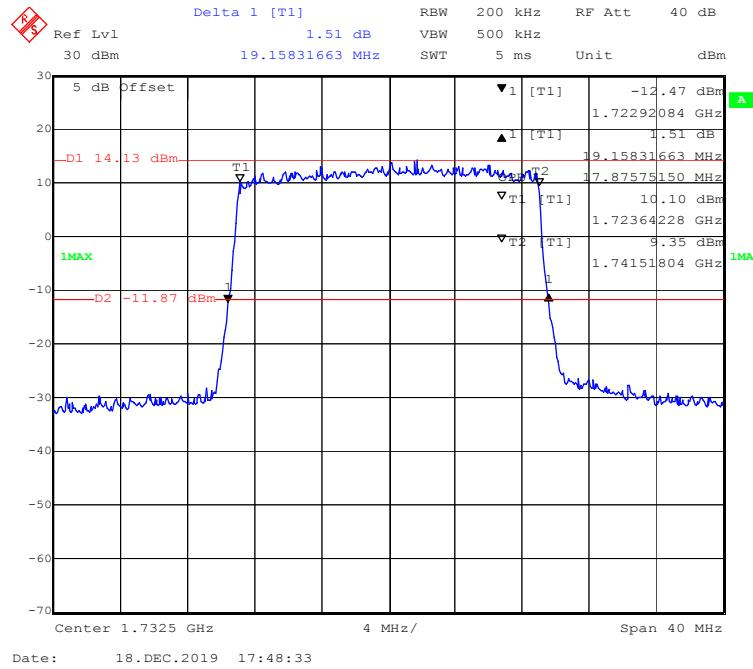
**16-QAM (1.4 MHz) - 99% Occupied & 26 dB Emissions Bandwidth, Middle channel**
