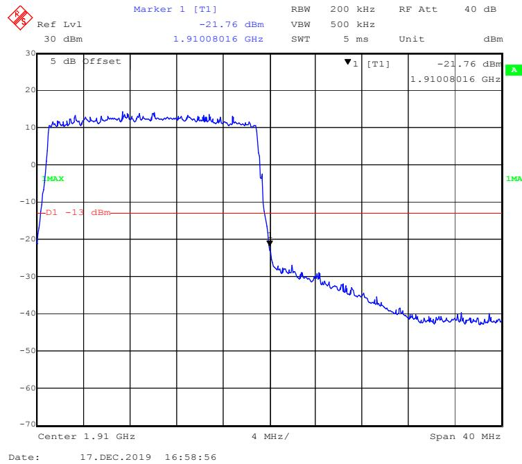
**16-QAM (1.4 MHz, FULL RB) - Left Band Edge**
