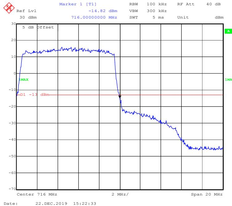
**16-QAM (1.4 MHz, FULL RB) - Left Band Edge**
