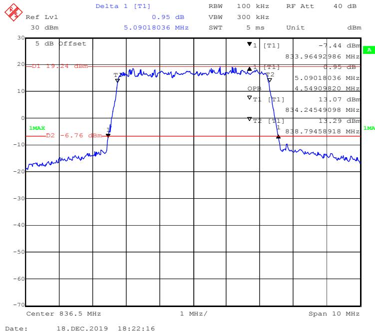
**QPSK (10MHz) - 99% Occupied & 26 dB Emissions Bandwidth, Middle channel**
