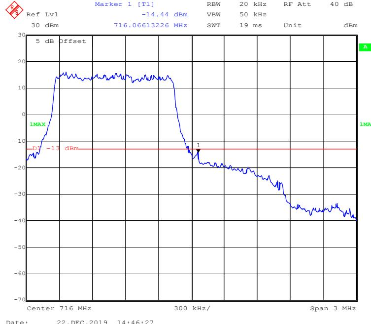
**QPSK (3 MHz, FULL RB) - Left Band Edge**
