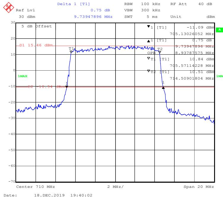
**16-QAM (5MHz) - 99% Occupied & 26 dB Emissions Bandwidth, Middle channel**
