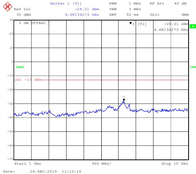
**LTE Band 17:****30 MHz - 1 GHz (5 MHz, QPSK, Middle Channel)**
