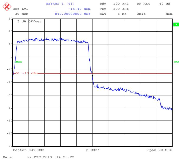
**16-QAM (1.4 MHz, FULL RB) - Left Band Edge**
