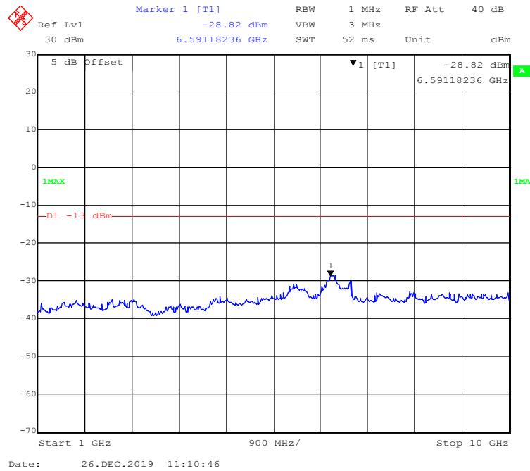
**30 MHz - 1 GHz (5 MHz, QPSK, Middle Channel)**
