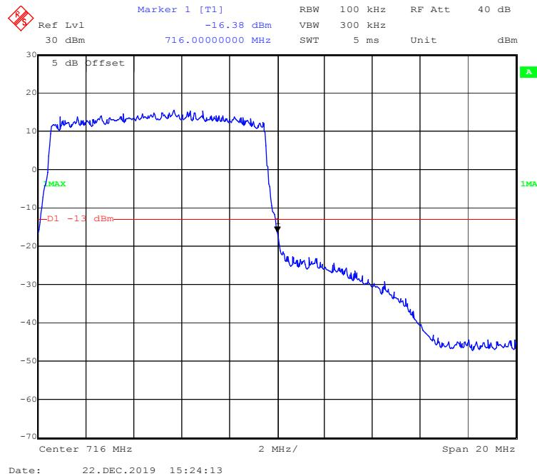
**LTE Band 17:****QPSK (5 MHz, FULL RB) - Left Band Edge**
