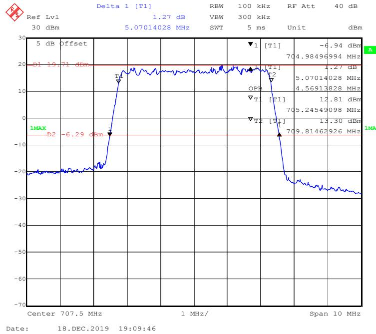
**QPSK (10MHz) - 99% Occupied & 26 dB Emissions Bandwidth, Middle channel**
