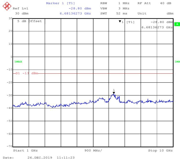
**30 MHz - 1 GHz (10 MHz, QPSK, Middle Channel)**
