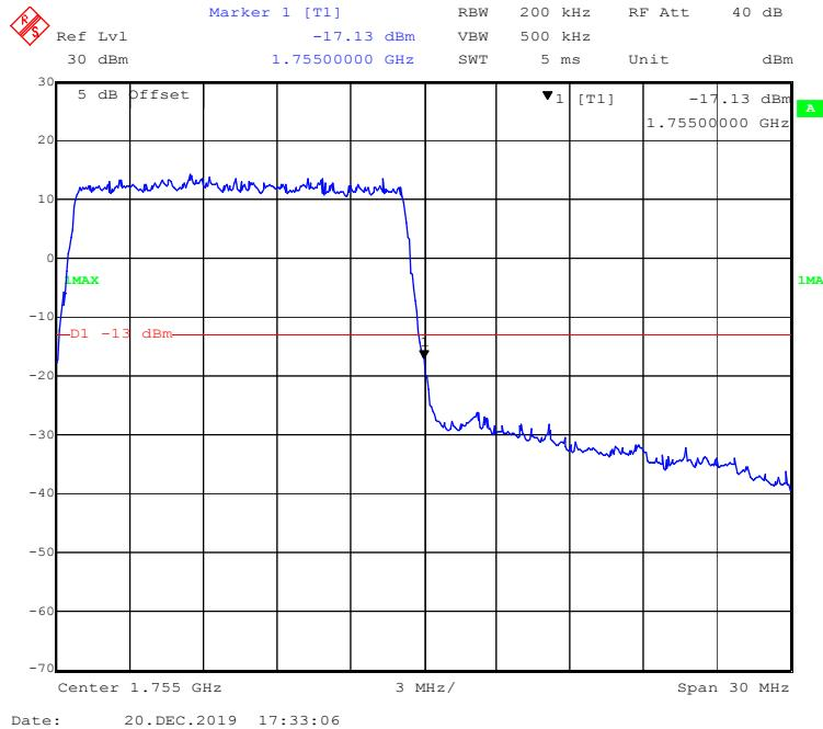
**QPSK (20 MHz, FULL RB) - Left Band Edge**
