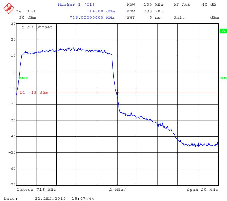
**16-QAM (5 MHz, FULL RB) - Left Band Edge**
