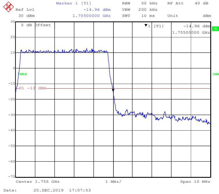
**QPSK (10 MHz, FULL RB) - Left Band Edge**
