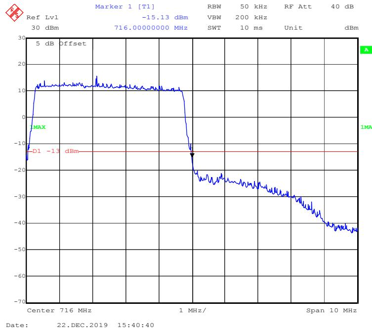
**16-QAM (10 MHz, FULL RB) - Left Band Edge**
