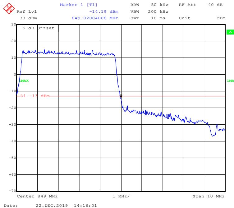
**QPSK (10 MHz, FULL RB) - Left Band Edge**
