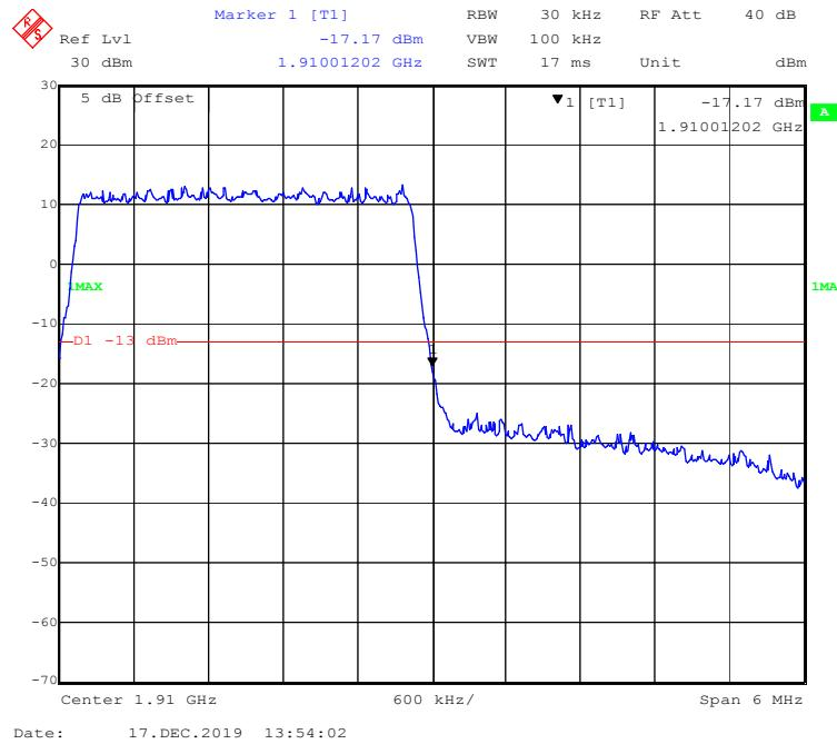
**16-QAM (5 MHz, FULL RB) - Left Band Edge**
