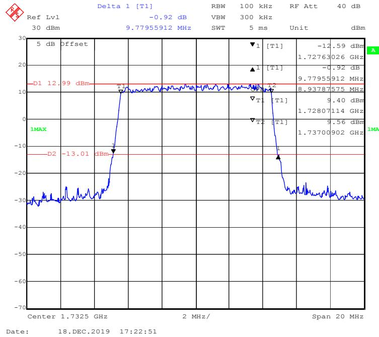
**16-QAM (15 MHz) - 99% Occupied & 26 dB Emissions Bandwidth, Middle channel**
