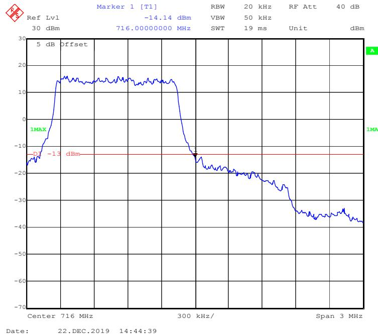
**16-QAM (3 MHz, FULL RB) - Left Band Edge**
