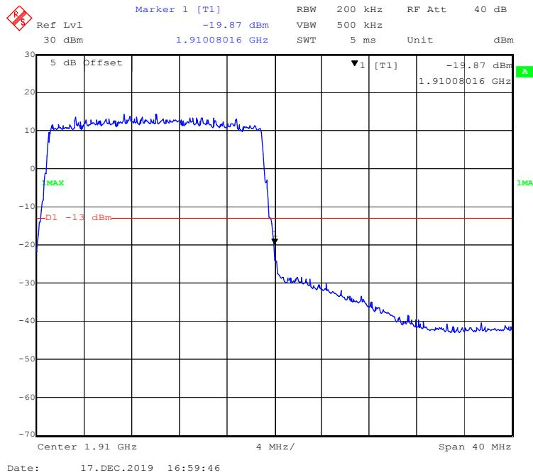
**LTE Band 4:****QPSK (1.4 MHz, FULL RB) - Left Band Edge**
