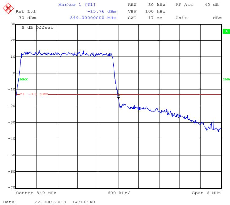
**16-QAM (5 MHz, FULL RB) - Left Band Edge**
