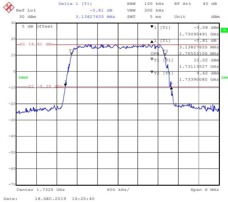
**16-QAM (5 MHz) - 99% Occupied & 26 dB Emissions Bandwidth, Middle channel**
