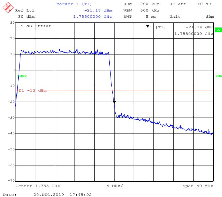
**16-QAM (1.4 MHz, FULL RB) - Left Band Edge**
