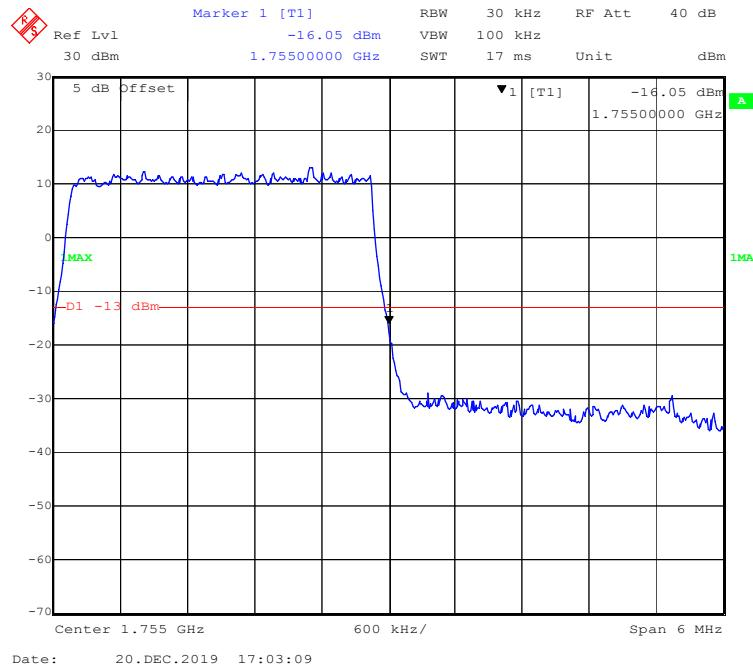
**QPSK (5 MHz, FULL RB) - Left Band Edge**
