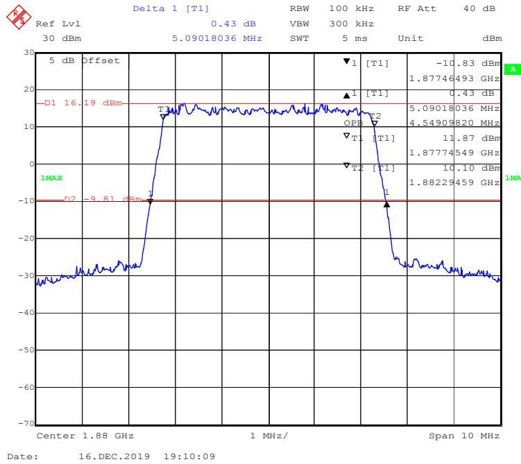
**QPSK (10MHz) - 99% Occupied & 26 dB Emissions Bandwidth, Middle channel**
