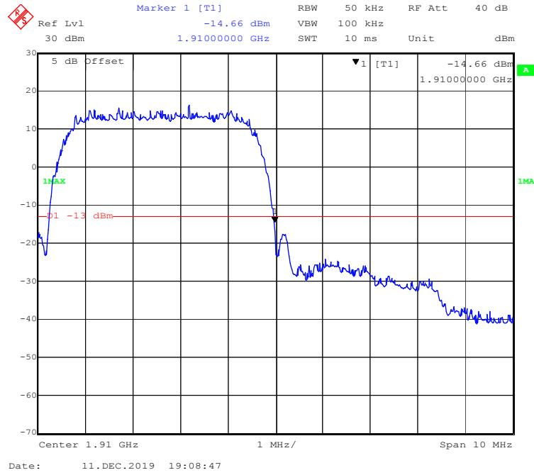
**LTE Band 2:****QPSK (1.4 MHz, FULL RB) - Left Band Edge**
