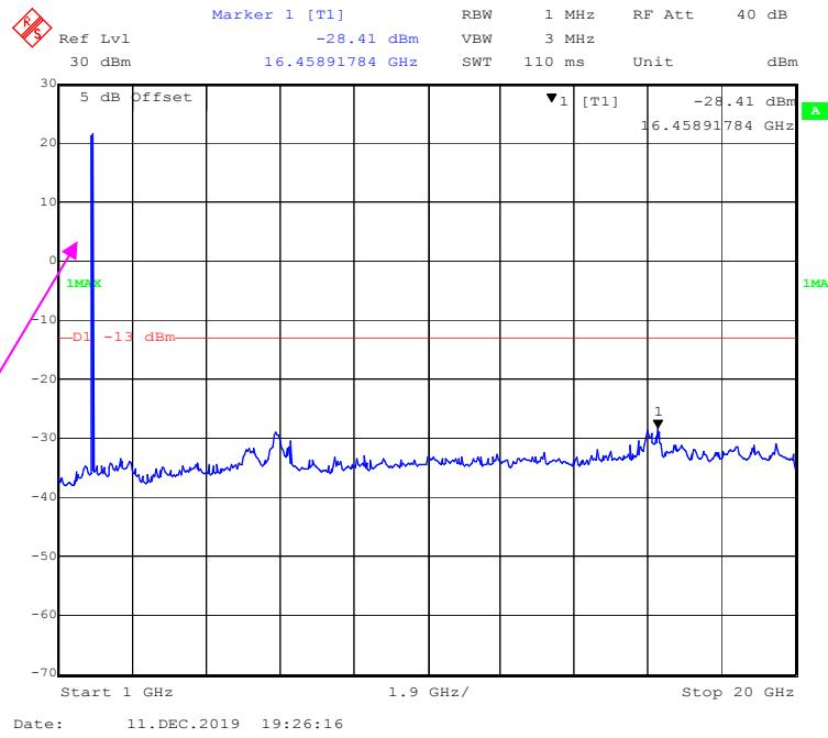
**30 MHz – 1GHz WCDMA (HSUPA) Mode, Middle channel**
