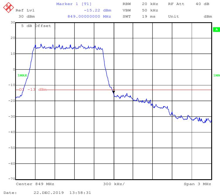
**16-QAM (3 MHz, FULL RB) - Left Band Edge**
