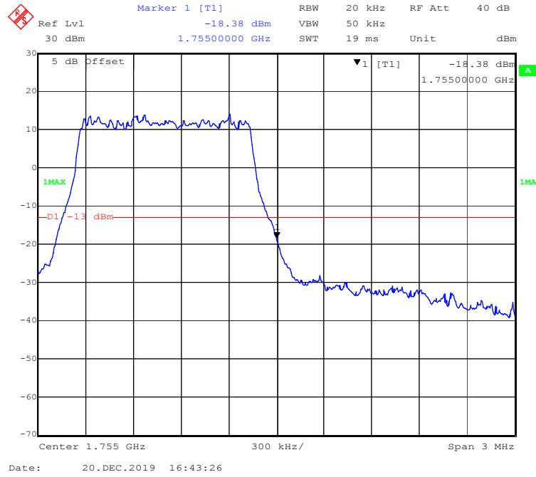
**16-QAM (3 MHz, FULL RB) - Left Band Edge**
