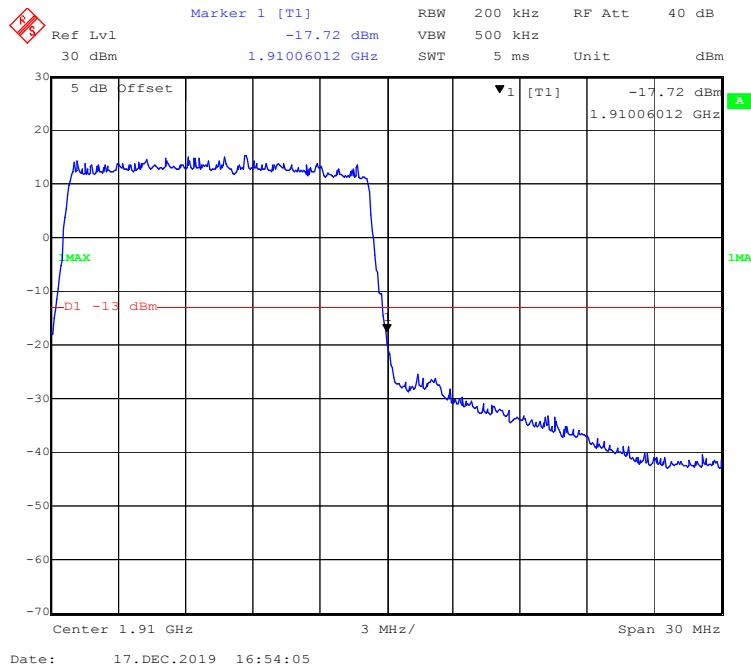
**QPSK (20 MHz, FULL RB) - Left Band Edge**
