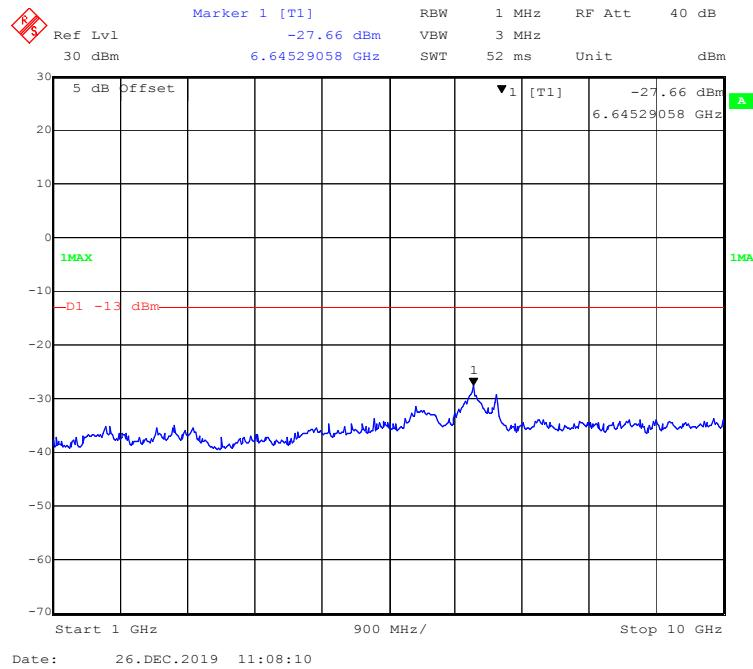
**LTE Band 12:****30 MHz - 1 GHz (1.4 MHz, QPSK, Middle Channel)**
