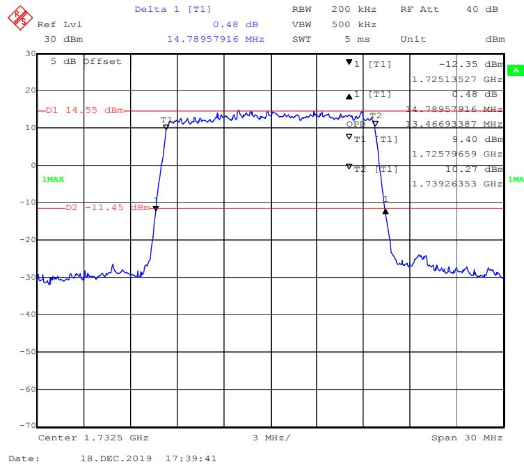
**16-QAM (20 MHz) - 99% Occupied & 26 dB Emissions Bandwidth, Middle channel**
