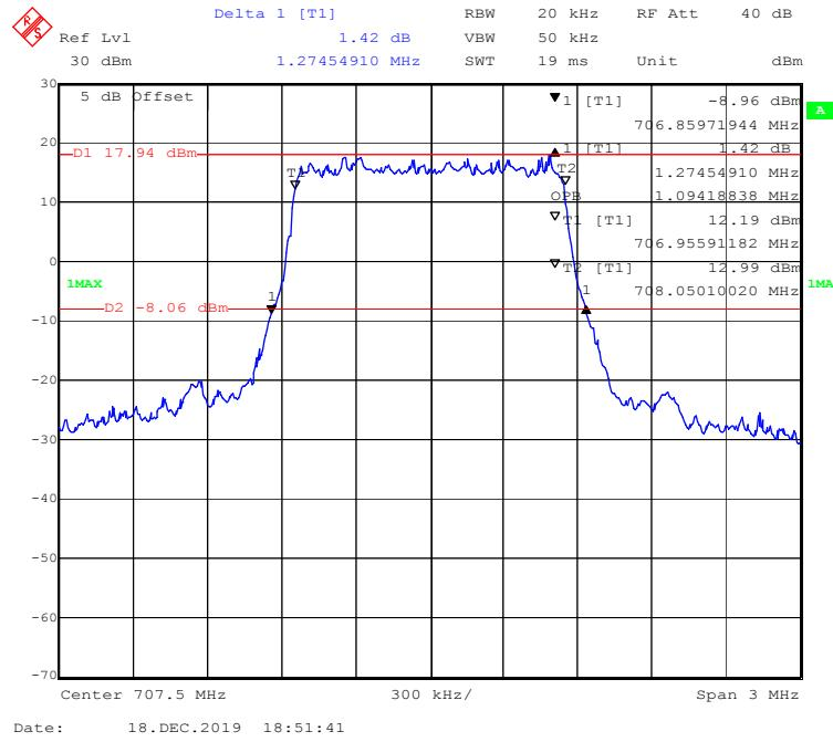
**QPSK (3 MHz) - 99% Occupied & 26 dB Emissions Bandwidth, Middle channel**
