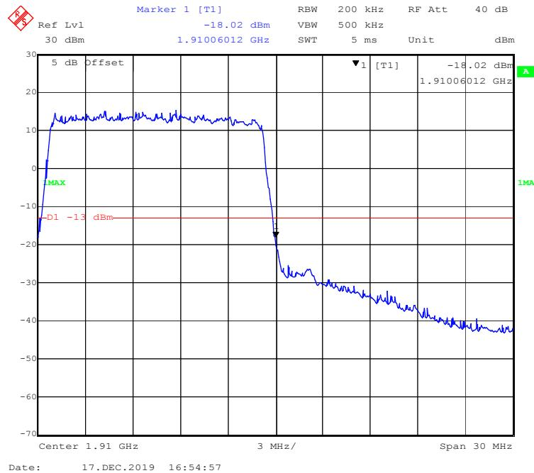
**16-QAM (20 MHz, FULL RB) - Left Band Edge**
