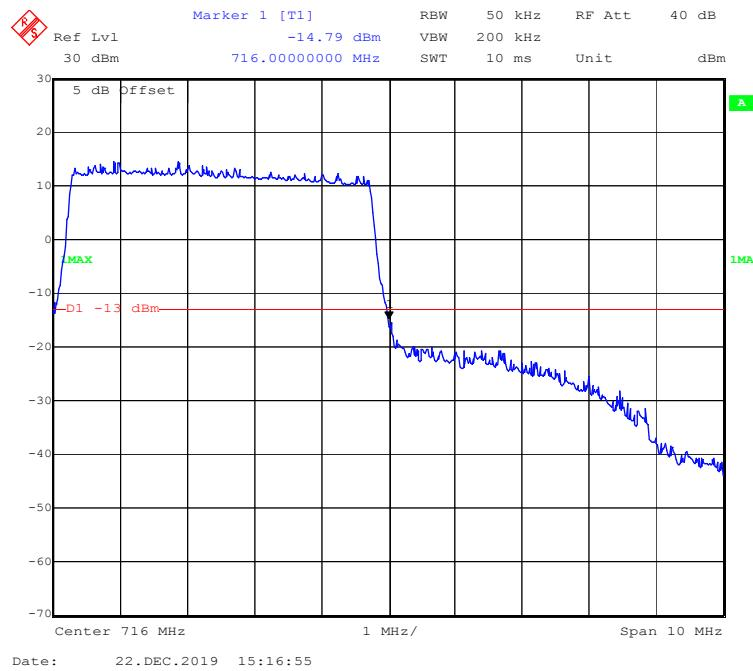
**QPSK (10 MHz, FULL RB) - Left Band Edge**
