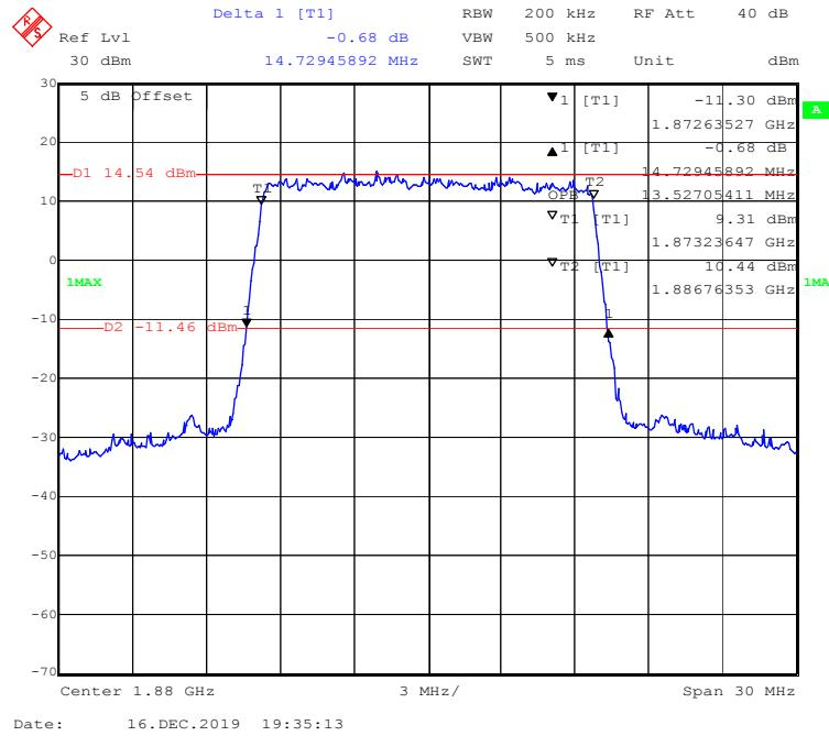
**16-QAM (20 MHz) - 99% Occupied & 26 dB Emissions Bandwidth, Middle channel**
