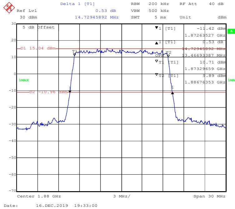
**QPSK (20 MHz) - 99% Occupied & 26 dB Emissions Bandwidth, Middle channel**
