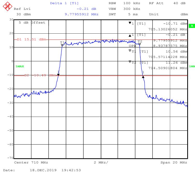
**FCC § 2.1051; § 22.917 (a); § 24.238 (a); §27.53(g) (h) - SPURIOUS EMISSIONS AT ANTENNA TERMINALS****Applicable Standards**
