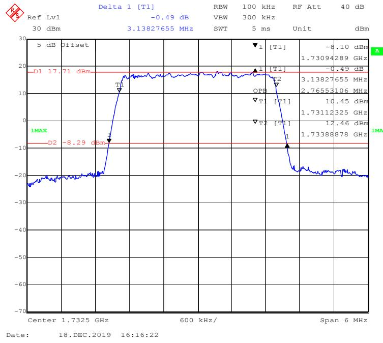
**QPSK (5MHz) - 99% Occupied & 26 dB Emissions Bandwidth, Middle channel**
