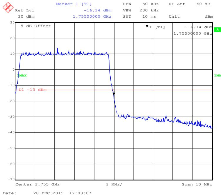
**16-QAM (10 MHz, FULL RB) - Left Band Edge**
