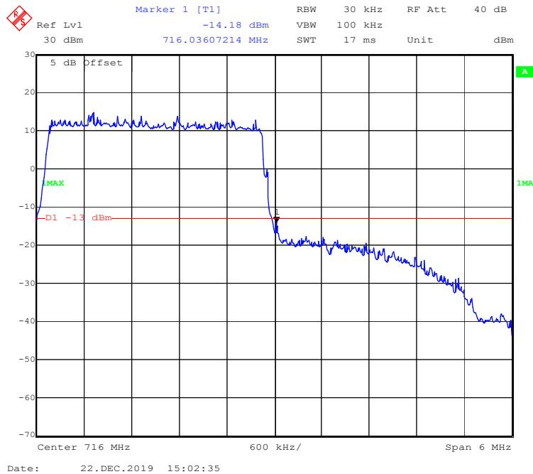
**16-QAM (5 MHz, FULL RB) - Left Band Edge**
