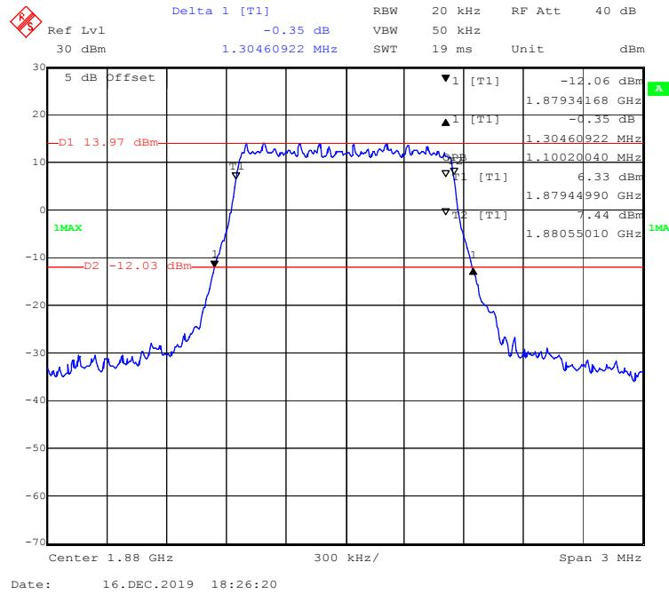
**16-QAM (3 MHz) - 99% Occupied & 26 dB Emissions Bandwidth, Middle channel**
