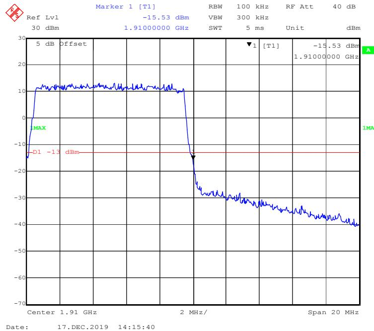
**16-QAM (15 MHz, FULL RB) - Left Band Edge**
