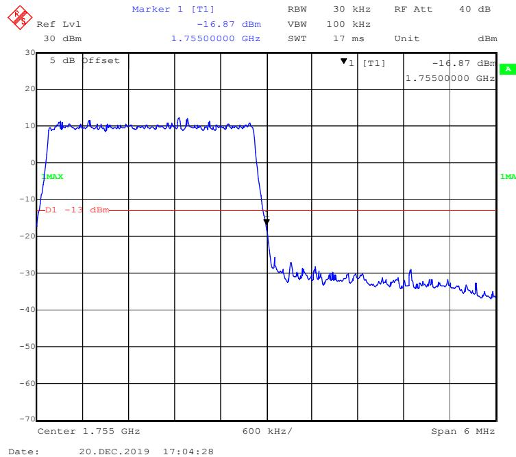
**16-QAM (5 MHz, FULL RB) - Left Band Edge**
