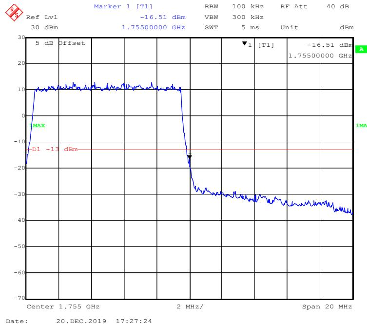
**QPSK (15 MHz, FULL RB) - Left Band Edge**
