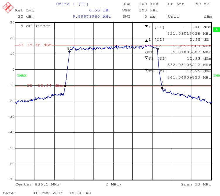
**16-QAM (1.4 MHz) - 99% Occupied & 26 dB Emissions Bandwidth, Middle channel**
