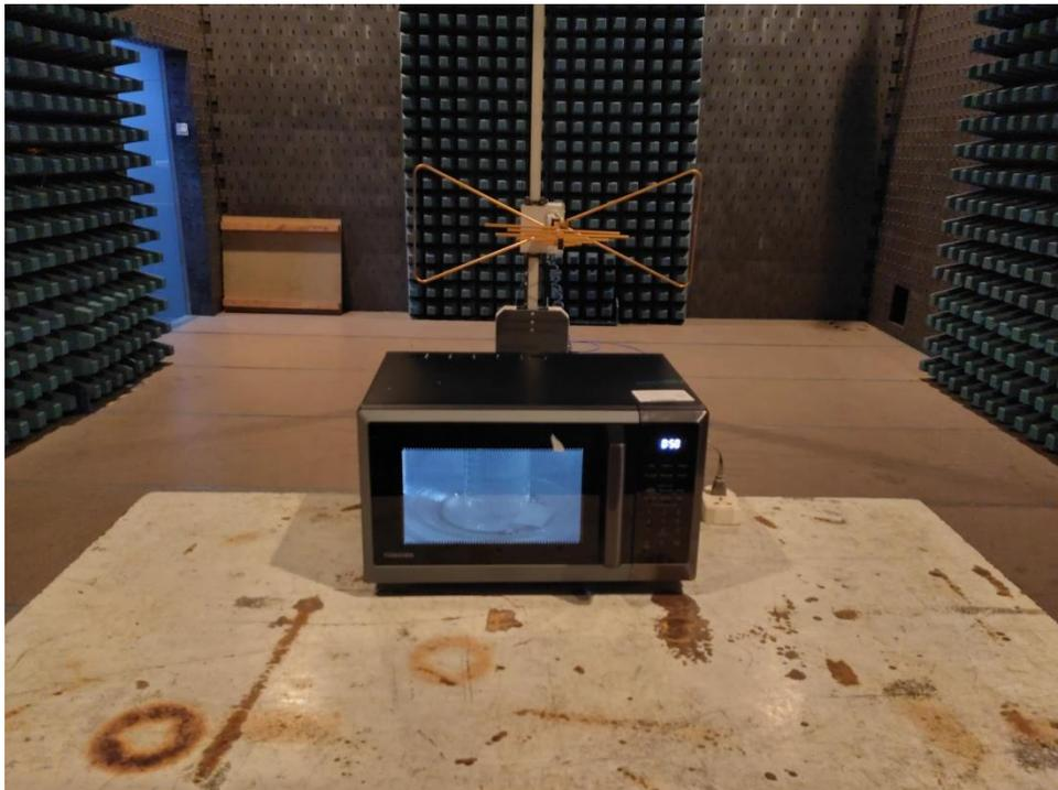
***Radiated Emission Test Set-up (1-25GHz):***
