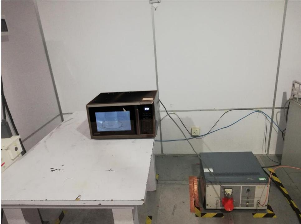
***Radiated Emission Test Set-up (30 -1,000MHz):***
