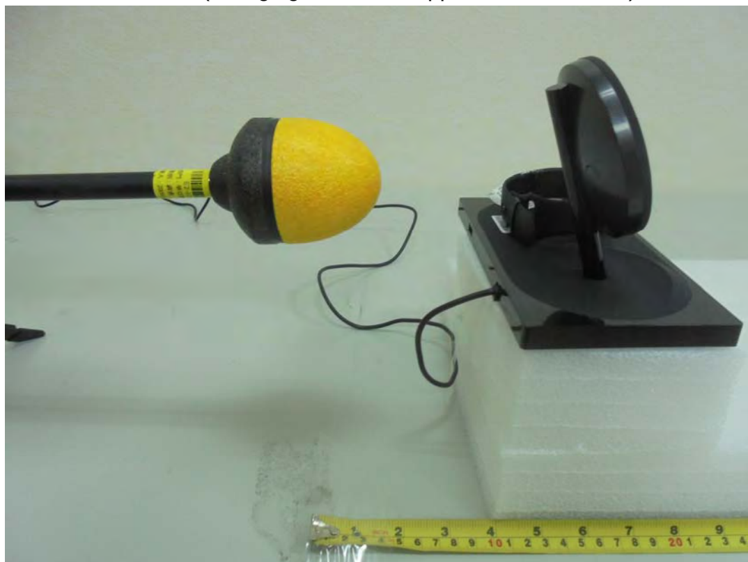
E-Field (Charging Mode with Apple Watch - Bottom)
