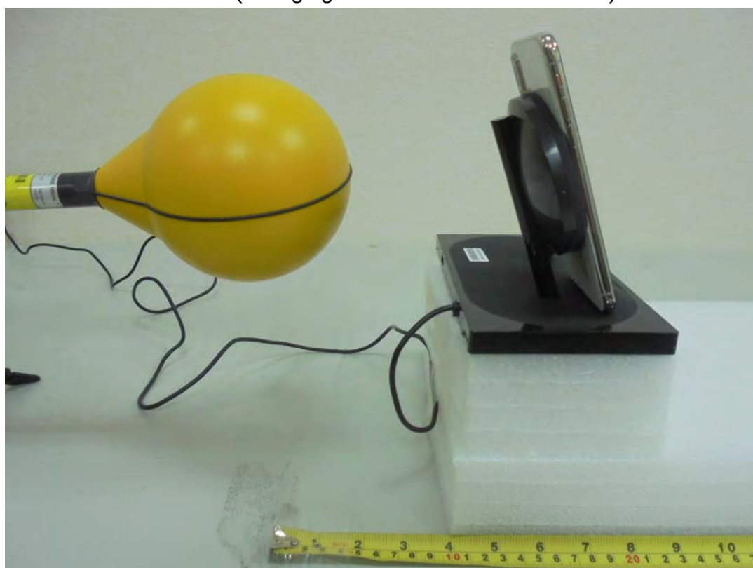
H -Field (Charging Mode with iPhone - Bottom)
