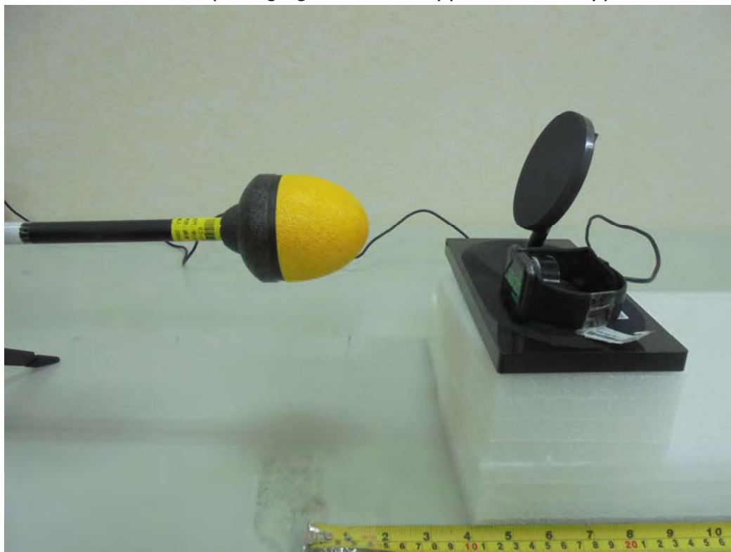
E-Field (Charging Mode with Apple Watch - Top)
