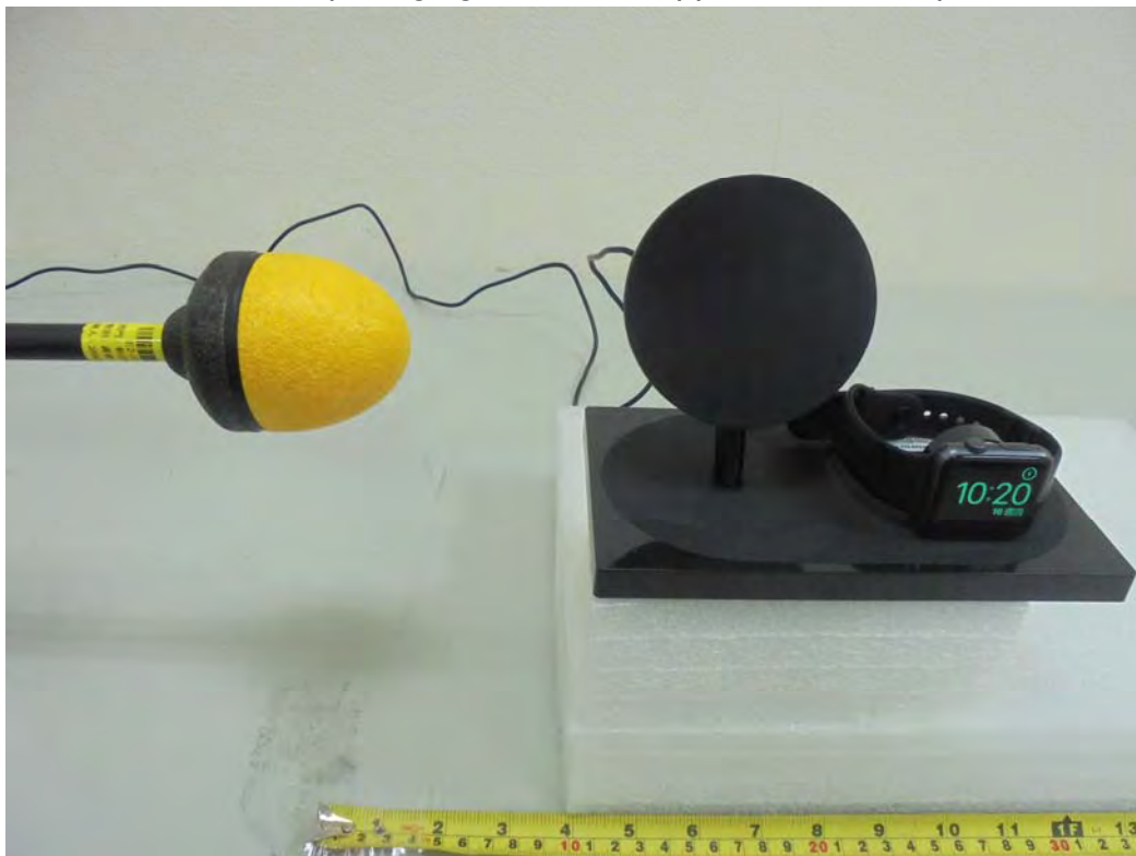
E-Field (Charging Mode with Apple Watch - Left)
