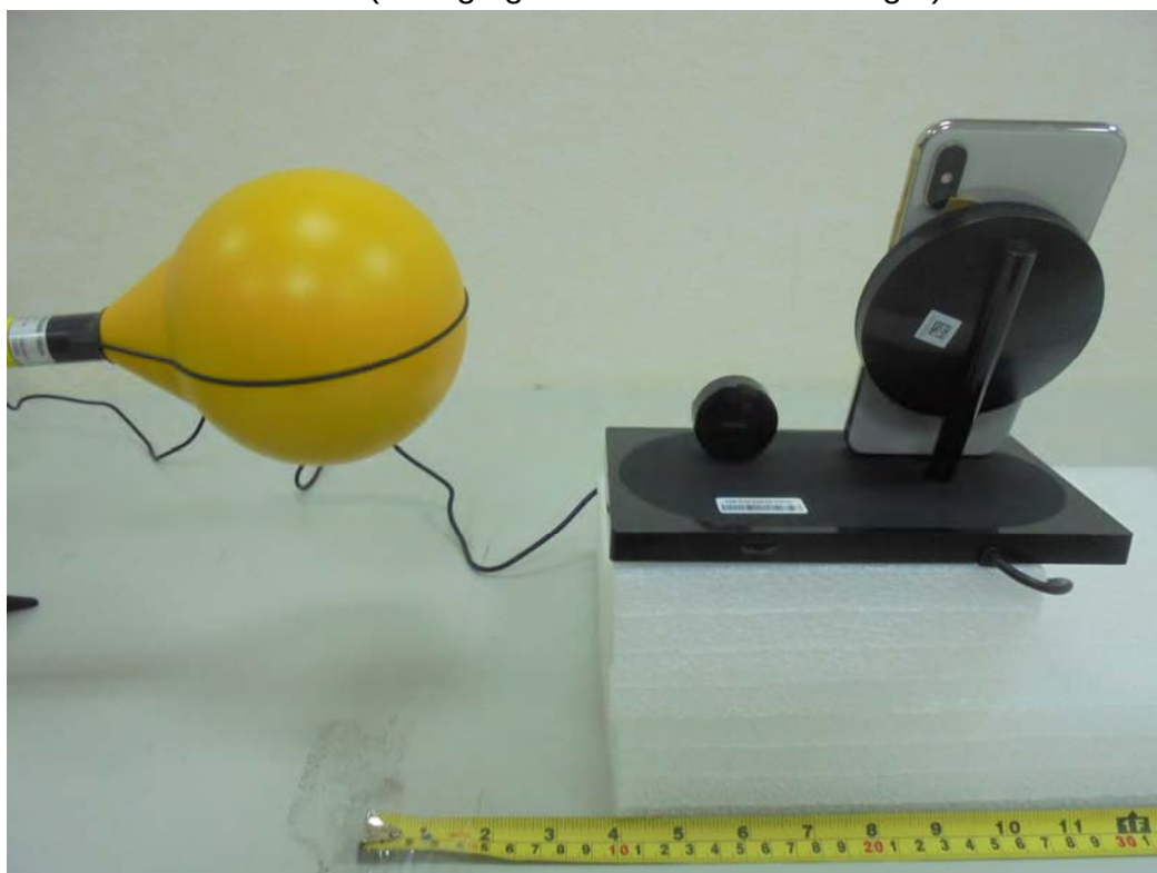
H -Field (Charging Mode with iPhone - Right)
