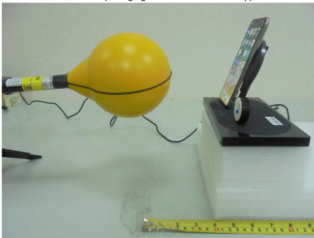
H -Field (Charging Mode with iPhone - Top)
