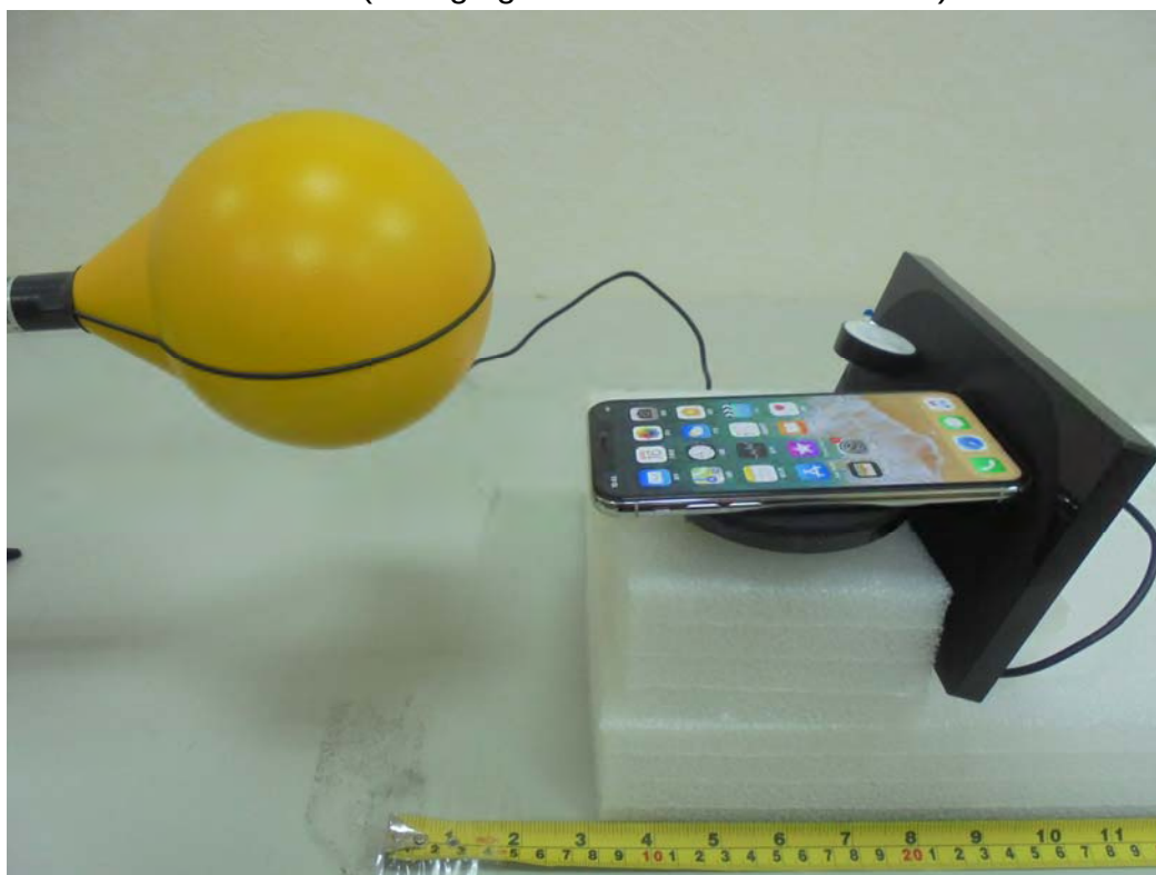
H -Field (Charging Mode with iPhone - Z-axis)
