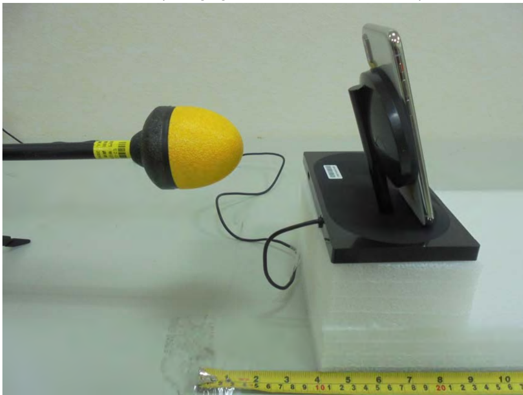
E-Field (Charging Mode with iPhone - Bottom)
