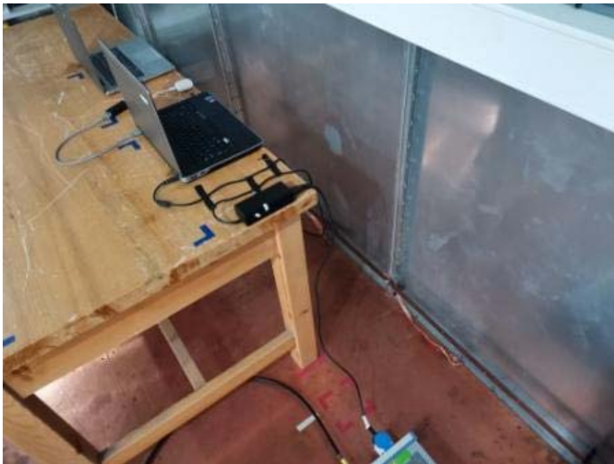
Conducted Emissions Test Setup (with charger)
