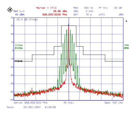
Plot # 34 Emission Mask B (Voice), Low Power, Freq. 866.00 MHz FM Modulation with 2.5 kHz Sine wave signal, 25 kHz Channel Spacing
