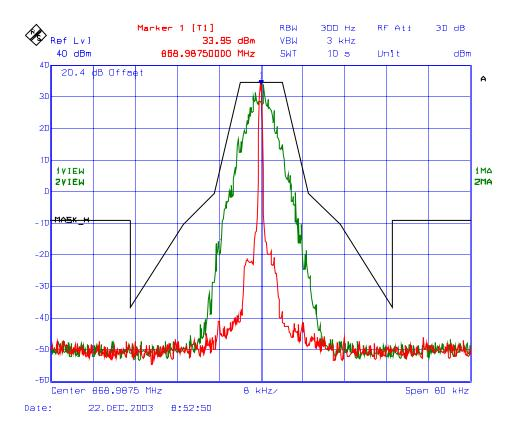
Plot # 39 Emission Mask H (Data), Low Power, Freq. 821.00 MHz
