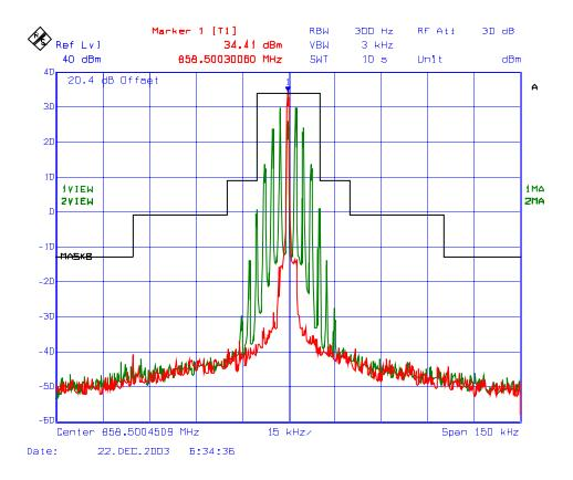
Plot # 28 Emission Mask B (Voice), High Power, Freq. 866.00 MHz FM Modulation with 2.5 kHz Sine wave signal, 25 kHz Channel Spacing
