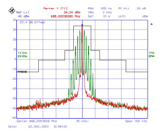
Plot # 29 Emission Mask B (Voice), Low Power, Freq. 806.00 MHz FM Modulation with 2.5 kHz Sine wave signal, 25 kHz Channel Spacing
