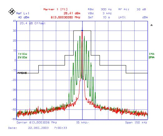
Plot # 31 Emission Mask B (Voice), Low Power, Freq. 821.00 MHz FM Modulation with 2.5 kHz Sine wave signal, 25 kHz Channel Spacing
