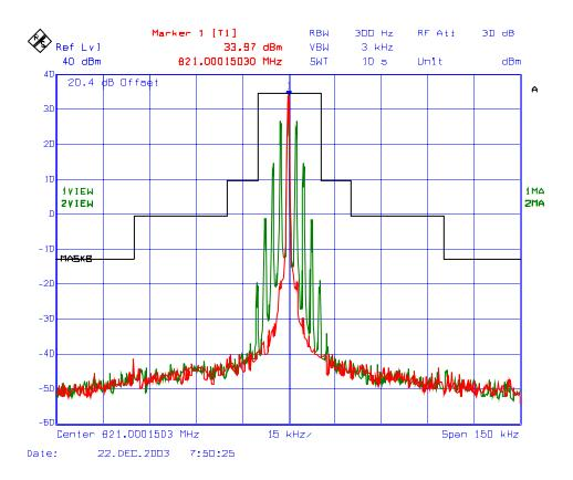
Plot # 16 Emission Mask B (Voice), High Power, Freq. 823.9875 MHz FM Modulation with 2.5 kHz Sine wave signal, 12.5 kHz Channel Spacing
