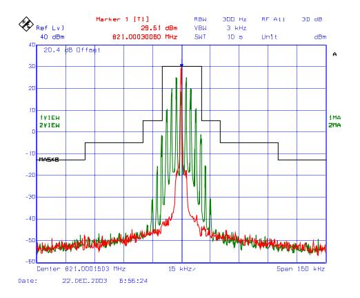
Plot # 32 Emission Mask B (Voice), Low Power, Freq. 851.0125 MHz FM Modulation with 2.5 kHz Sine wave signal, 25 kHz Channel Spacing
