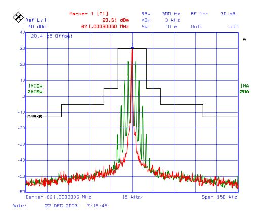
Plot # 20 Emission Mask B (Voice), Low Power, Freq. 823.9875 MHz FM Modulation with 2.5 kHz Sine wave signal, 12.5 kHz Channel Spacing
