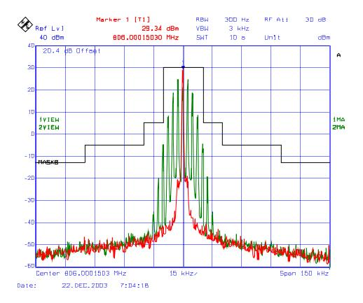
Plot # 30 Emission Mask B (Voice), Low Power, Freq. 813.50 MHz FM Modulation with 2.5 kHz Sine wave signal, 25 kHz Channel Spacing
