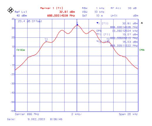
Plot #: 4 99% Occupied Bandwidth Measurement, Freq: 868.9875 MHz 12.5 kHz Channel Spacing, FM Modulation, 2.5 kHz Sine wave signal
