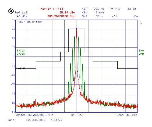
Plot # 23 Emission Mask B (Voice), High Power, Freq. 806.00 MHz FM Modulation with 2.5 kHz Sine wave signal, 25 kHz Channel Spacing
