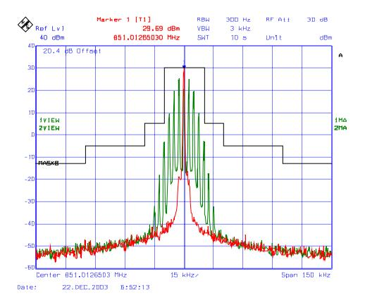
Plot # 33 Emission Mask B (Voice), Low Power, Freq. 858.50 MHz FM Modulation with 2.5 kHz Sine wave signal, 25 kHz Channel Spacing
