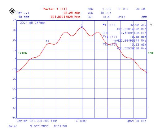
Plot #: 2 99% Occupied Bandwidth Measurement, Freq: 823.9875 MHz 12.5 kHz Channel Spacing, FM Modulation, 2.5 kHz Sine wave signal
