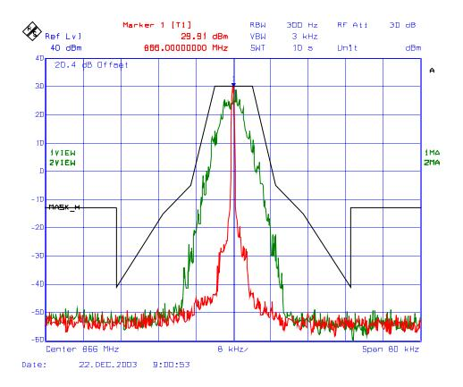
Plot # 42 Emission Mask H (Data), Low Power, Freq. 868.9875 MHz
