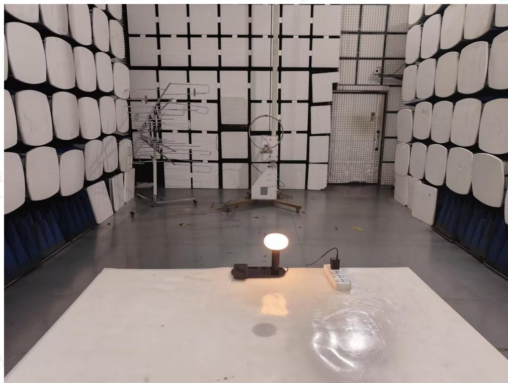
Radiated Emission below 30MHz-AC adapter charge mode
