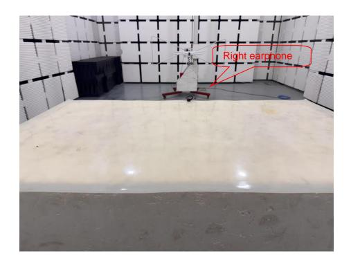
Set-up for Radiated Spurious Emission, Above 1GHz
