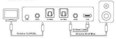
Use the BYPASS function if your TV only has ONE OPTICAL Output which is currently occupied by your AV receiver or sound bar Toggle between BYPASS and Bluetooth mode using a simple switch. No need to unplug cable. In Bypass mode, "BT5809" can be used as a decoder to convert audio between 3.5mm AUX and optical output.
