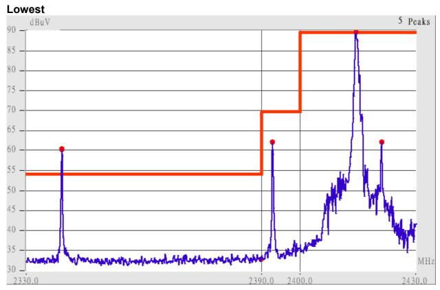
This is the hard copy of our bandedge measurement generated by our bandedge testing program. The plot shown above is the bandedge of lowest channel.
