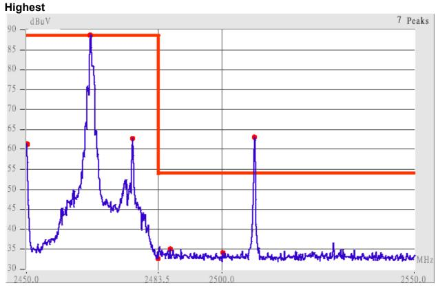
This is the hard copy of our bandedge measurement generated by our bandedge testing program. The plot shown above is the bandedge of highest channel.
