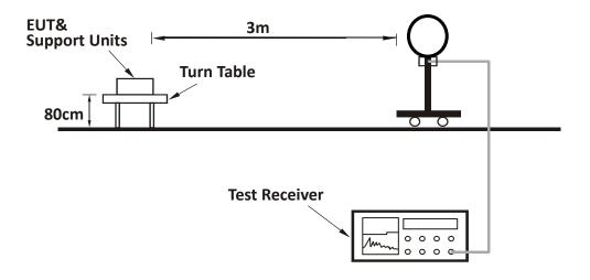
For Radiated emission 30MHz to 1GHz:
