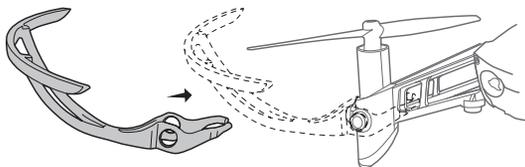
To remove the hulls: gently remove the hulls from the Parrot Mambo's contacts.
