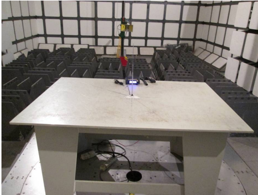
Radiated Emissions – Front View (Above 1 GHz)
