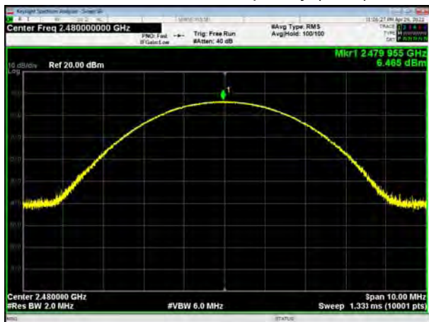
BT 3DH5 CH78, Carrier frequency (MHz): 2480
