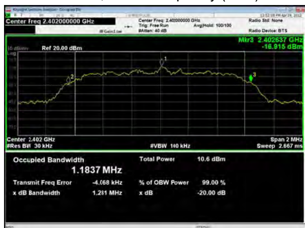
BT 2DH5 CH39, Carrier frequency (MHz): 2441
