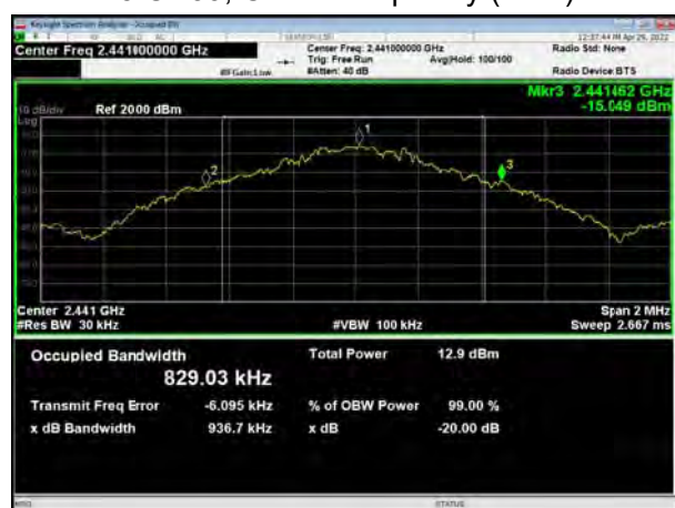
BT DH5 CH78, Carrier frequency (MHz): 2480
