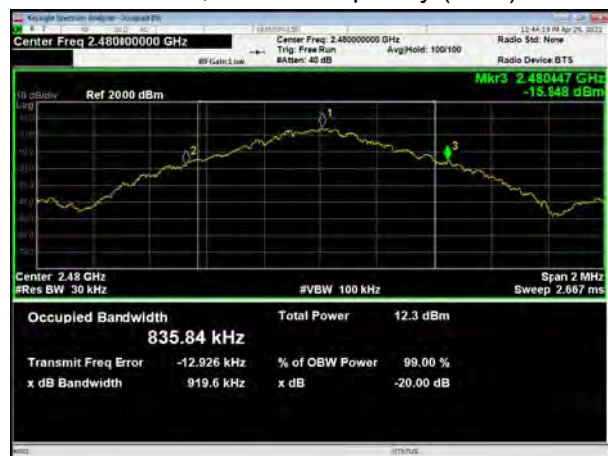
BT DH5 CH78, Carrier frequency (MHz): 2480
