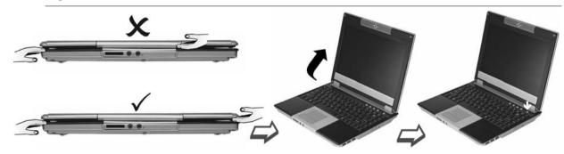
Raise the LCD panel and follow the correct procedures as shown on the illustration.
