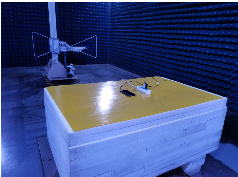
Photo of Radiated Emission Measurement (Above 1G)
