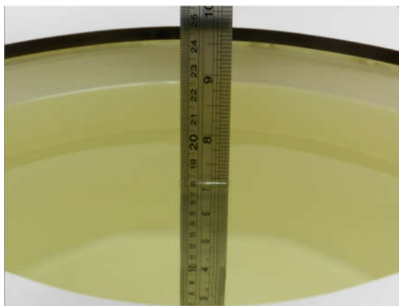
Fig 11.1 Photo of Liquid Height for Body SAR
