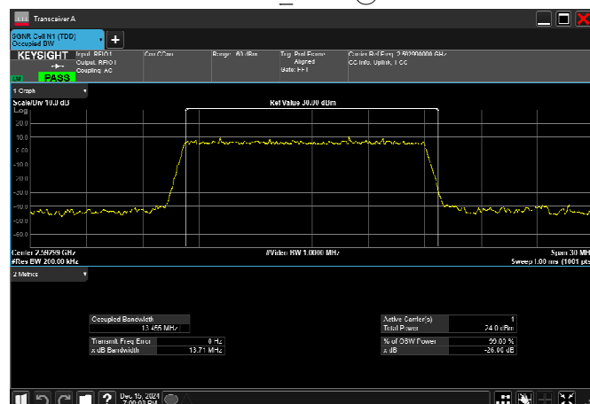
n41_15MHz_30kHz_2592.99MHz_DFT-s-OFDM 16 QAM RB36@0
