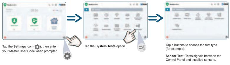
**Panel Test:** Tests the function of the Edge Panel's audio and buttons.
