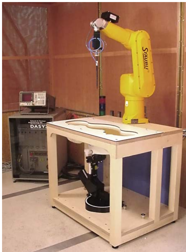
DASY3 SAR Measurement System with SAM phantom
