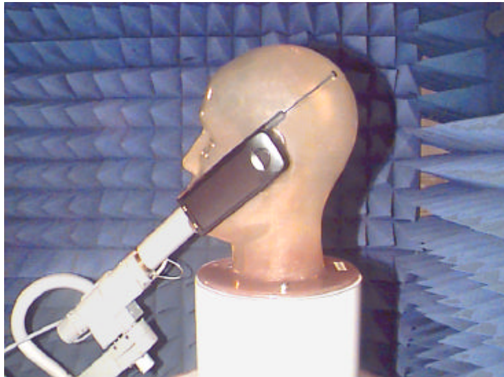
Figure 9. Sample of Handset alignment with the Ear Canal of the Phantom
