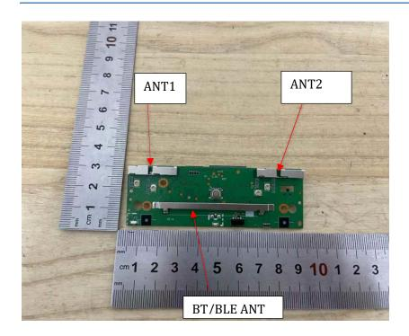
The four Connector in the photo are no use, there are only three PIFA antennas from this module
