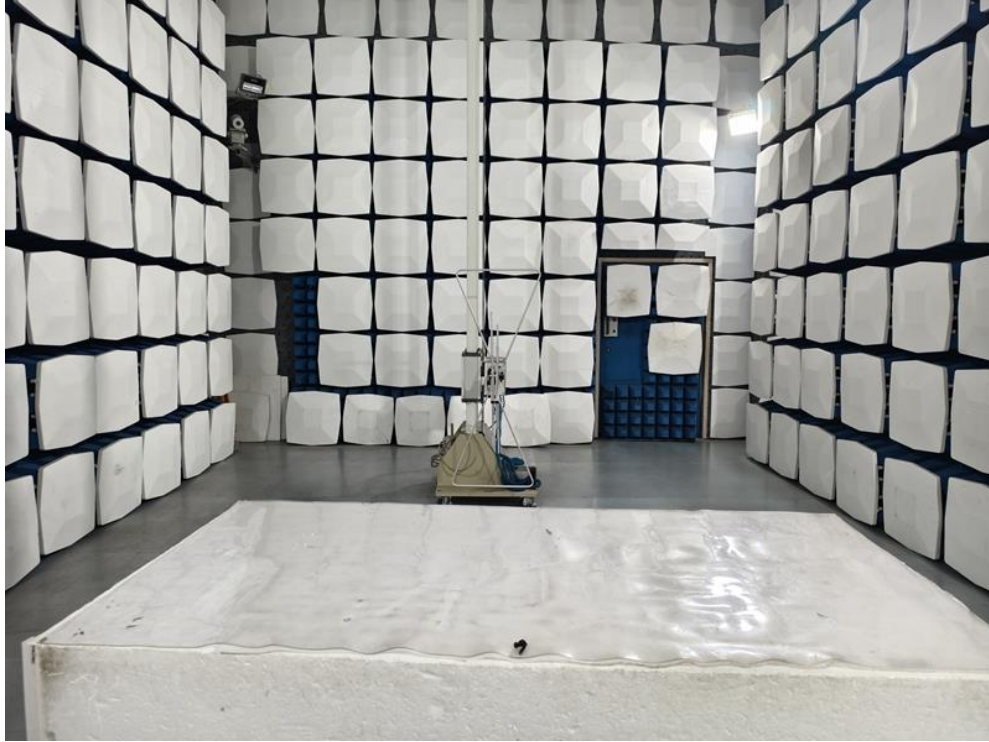
Radiated Emission Test Setup:
