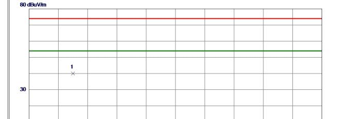
Reading Correct Measure No. Freq. Limit Margin Level Factor ment MHz dBuV/mdBuV/m $dBuV/m \quad dB$ Comment dΒ Detector 4824.0000 49.68 74.00 1 \* -9.69 39.99 -34.01Peak
