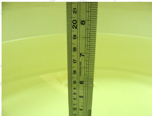
Photo of Liquid Height for Body SAR
