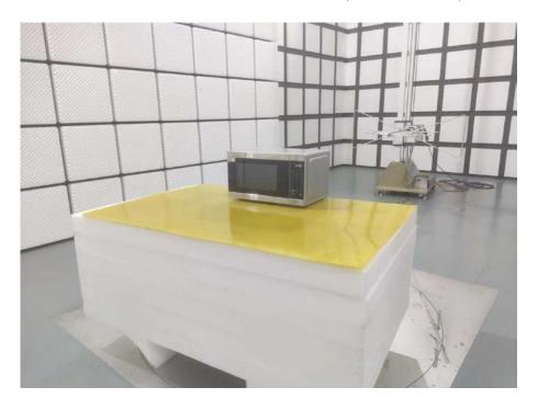
**Radiated Emissions Test View (Above 1GHz)**
