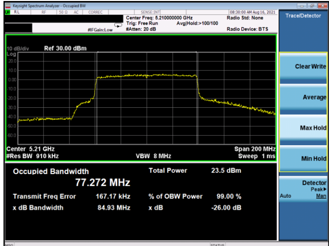
Plot 7-6. 26dB BW & 99% OBW Antenna 5T (80MHz BW 802.11ax(SU) – Ch. 42, MCS2)
