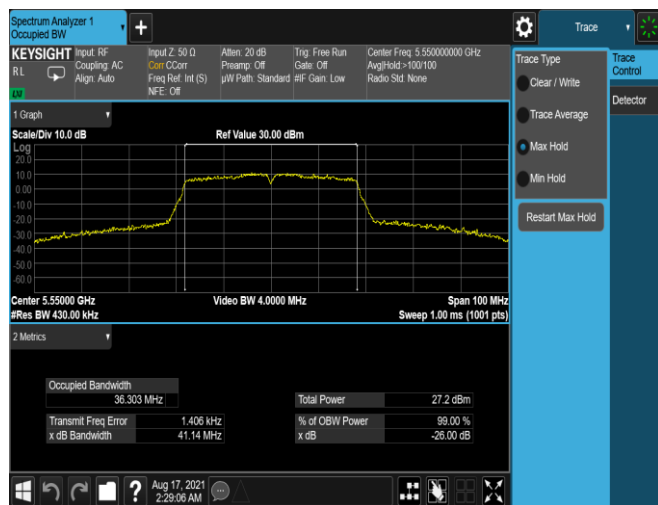
Plot 7-33. 26dB BW & 99% OBW Antenna 5T (40MHz BW 802.11n – Ch. 110, MCS3)
