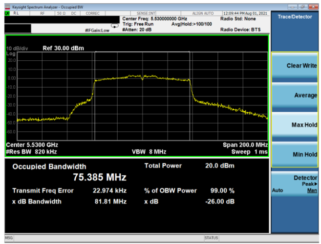
Plot 7-17. 26dB BW & 99% OBW Antenna 5T (80MHz BW 802.11ac - Ch. 106, MCS2)
