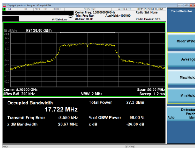
Plot 7-19. 26dB BW & 99% OBW Antenna 5T (20MHz BW 802.11n - Ch. 40, MCS3)
