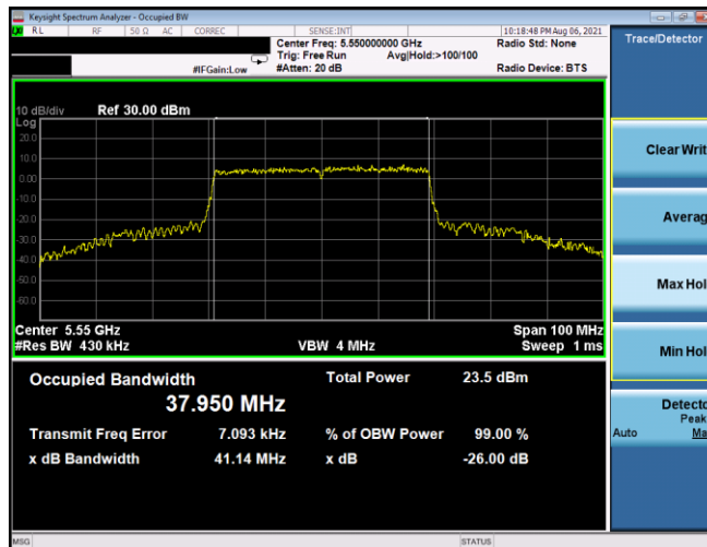
Plot 7-52. 26dB BW & 99% OBW Antenna 5T (40MHz BW 802.11ax(SU) – Ch. 110, MCS5)
