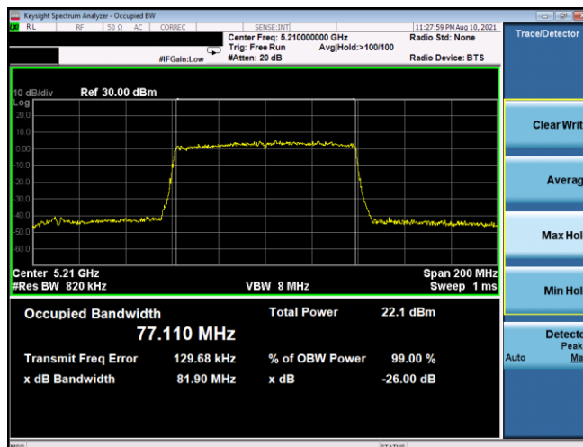
Plot 7-42. 26dB BW & 99% OBW Antenna 5T (80MHz BW 802.11ax(SU) – Ch. 42, MCS5)
