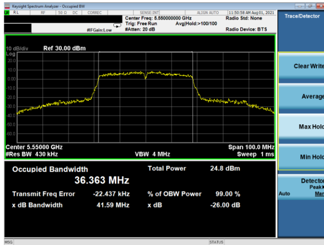
Plot 7-15. 26dB BW & 99% OBW Antenna 5T (40MHz BW 802.11n - Ch. 110, MCS2)
