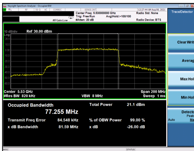
Plot 7-36. 26dB BW & 99% OBW Antenna 5T (80MHz BW 802.11ax(SU) – Ch. 106, MCS3)
