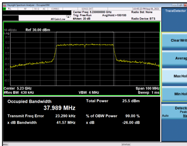
Plot 7-22. 26dB BW & 99% OBW Antenna 5T (40MHz BW 802.11ax(SU) - Ch. 46, MCS3)
