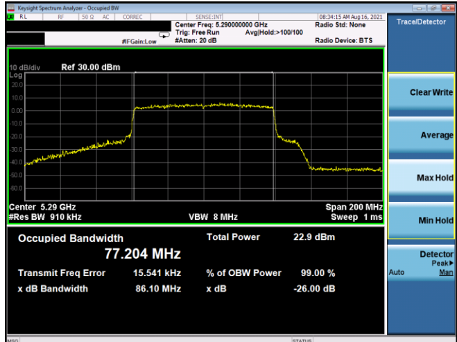
Plot 7-12. 26dB BW & 99% OBW Antenna 5T (80MHz BW 802.11ax(SU) – Ch. 58, MCS2)
