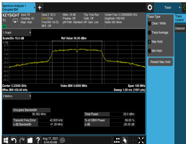
Plot 7-21. 26dB BW & 99% OBW Antenna 5T (40MHz BW 802.11n - Ch. 46, MCS3)
