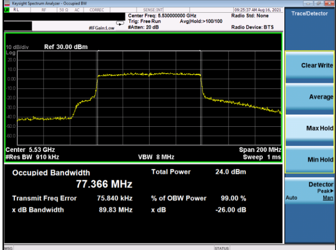
Plot 7-18. 26dB BW & 99% OBW Antenna 5T (80MHz BW 802.11ax(SU) - Ch. 106, MCS2)
