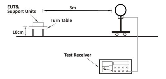
For Radiated emission 30MHz to 1GHz:
