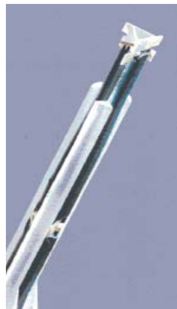
Inside view of ES3DV2 E-field Probe
