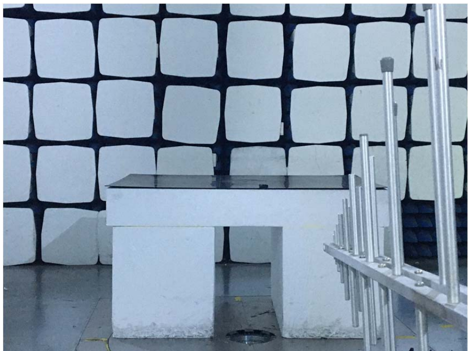
Radiation Emission Test Setup (30MHz to 1GHz)
