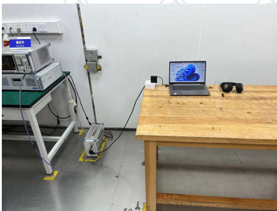
Conducted Emissions Test Setup
