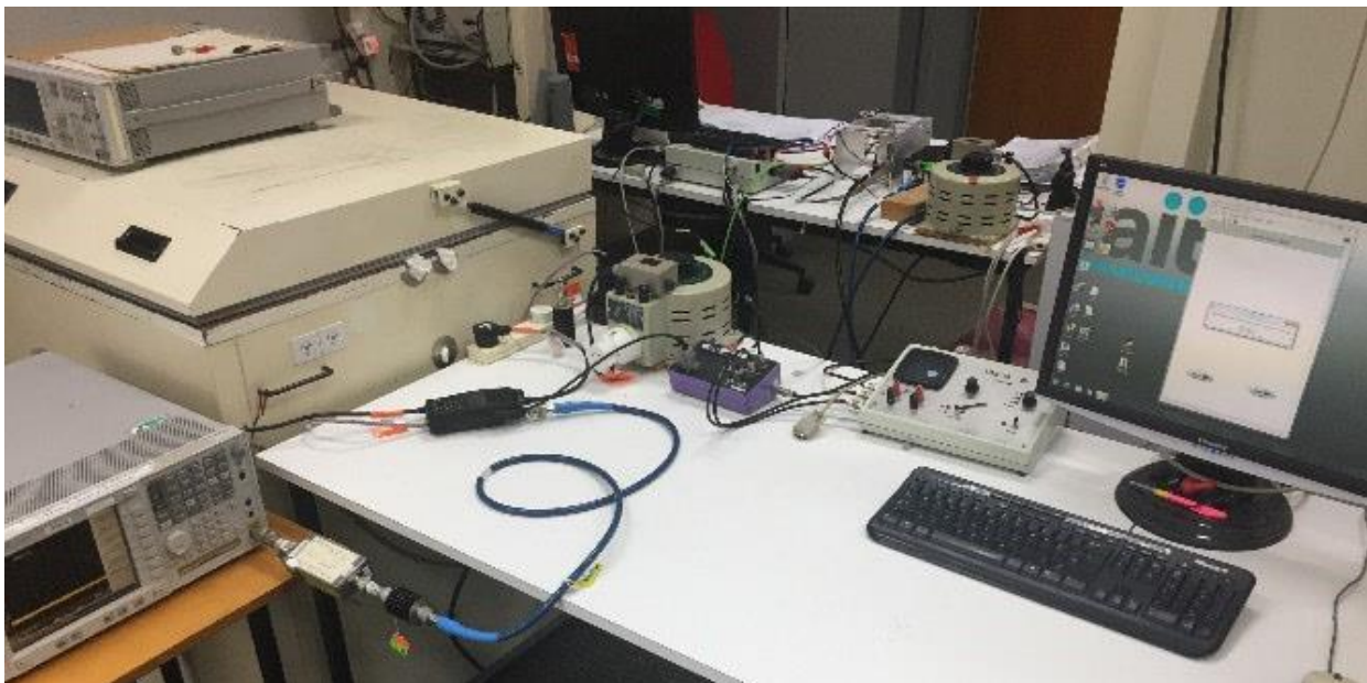
Photo: Conducted Emissions Test Setup
