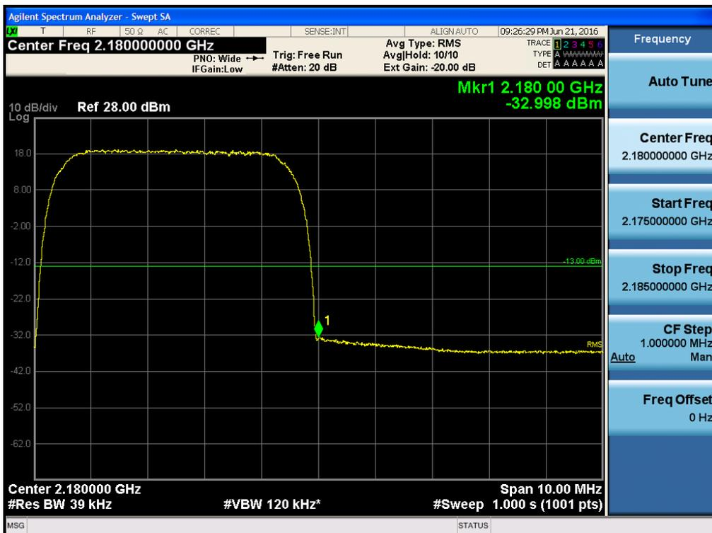
**Multi channel Enhancer Band Edge for IC\_AWS BAND**
