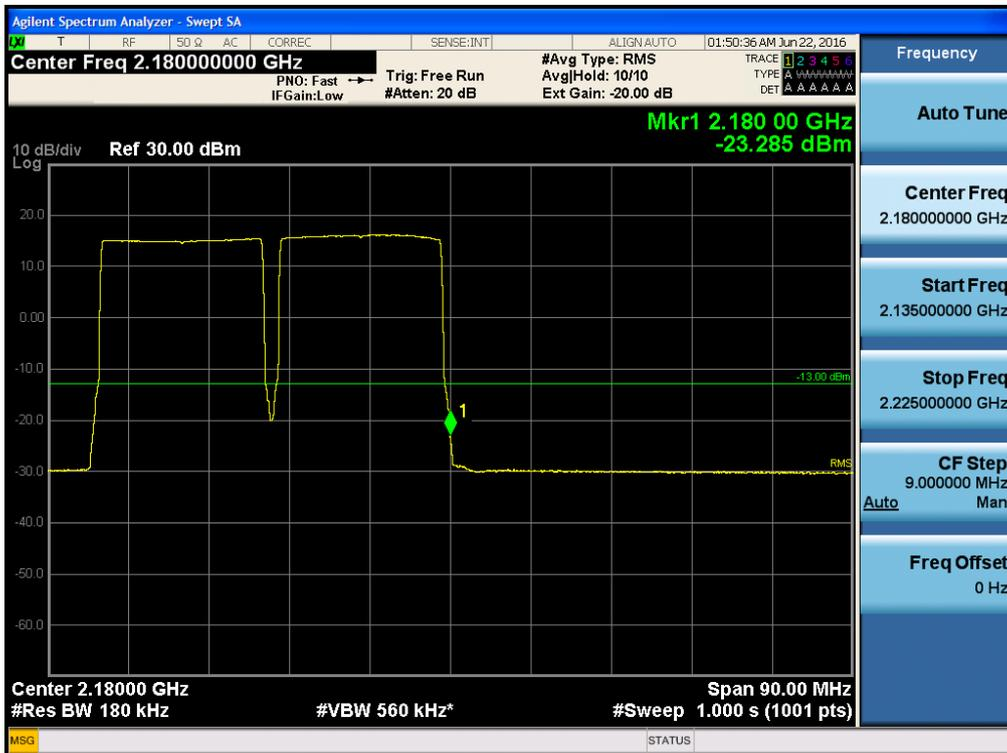
**Intermodulation Spurious Emissions for FCC\_AWS CDMA**
