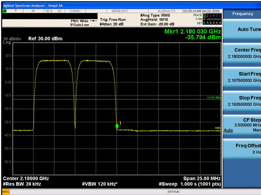
**Single channel Enhancer Band Edge\_AWS13 BAND LTE 5MHz**
