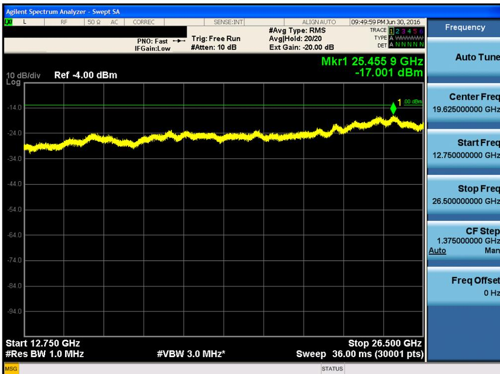
**Intermodulation Spurious Emissions for FCC\_AWSBAND LTE 5MHz**
