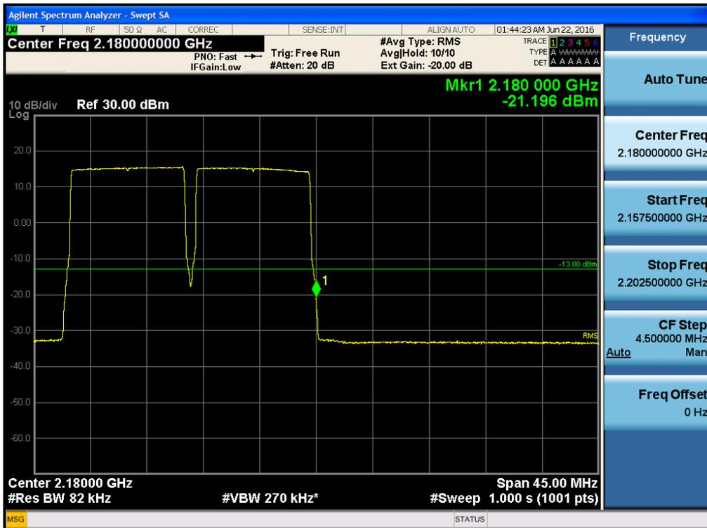
**Intermodulation Spurious Emissions for FCC\_AWSBAND LTE 20MHz**
