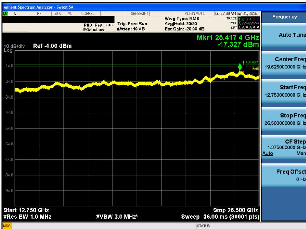
**Single channel Enhancer Plots of Spurious Emission for AWS BAND LTE 20MHz
