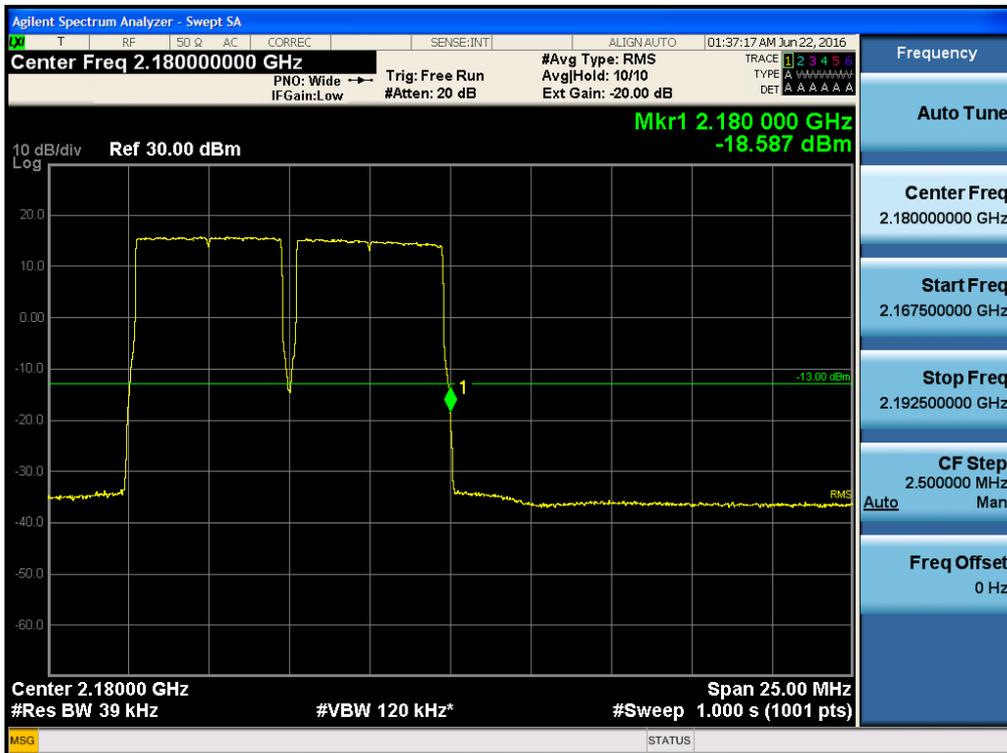
**Intermodulation Spurious Emissions for FCC\_AWSBAND LTE 10MHz**
