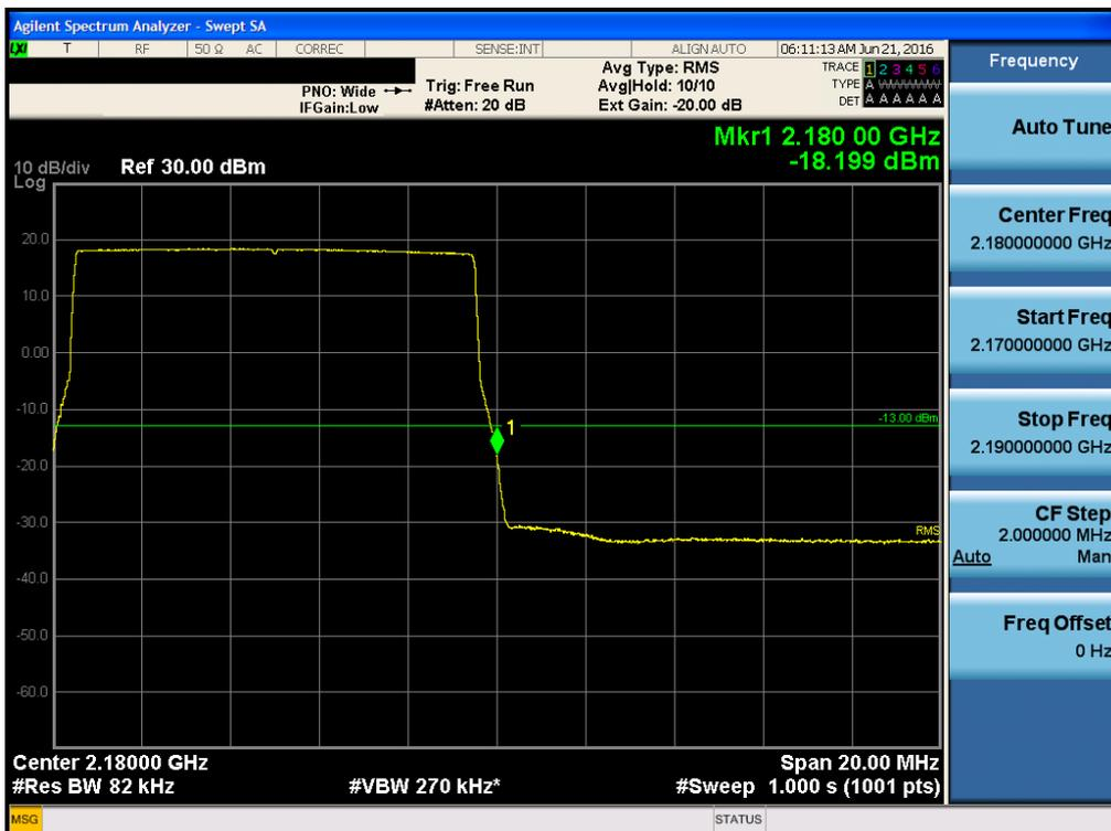
**Single channel Enhancer Band Edge\_AWS BAND LTE 20 MHz**
