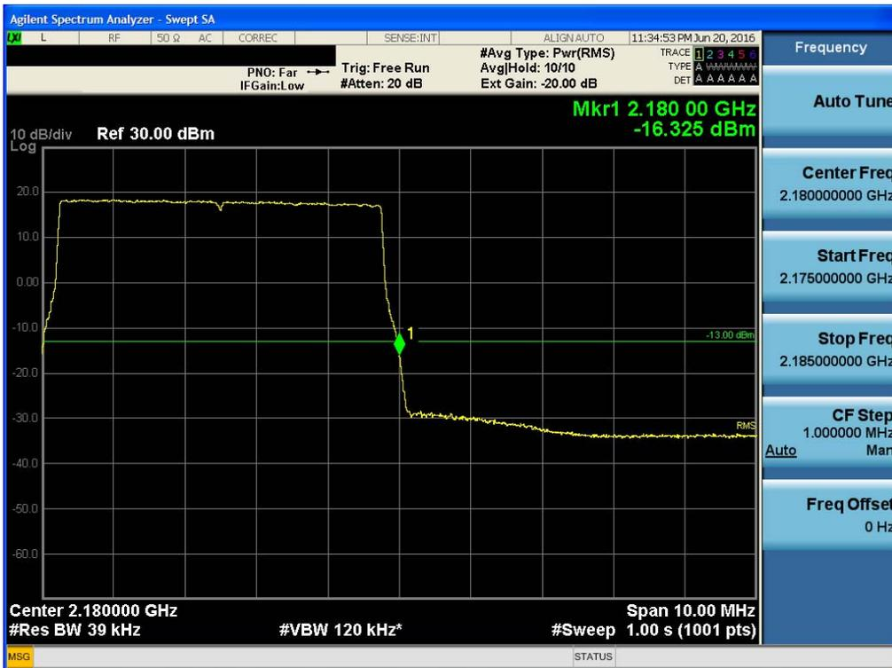
**Single channel Enhancer Band Edge\_AWS13 BAND LTE 10MHz**
