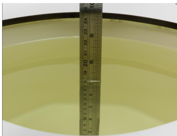
Fig 10.2 Photo of Liquid Height for Body SAR
