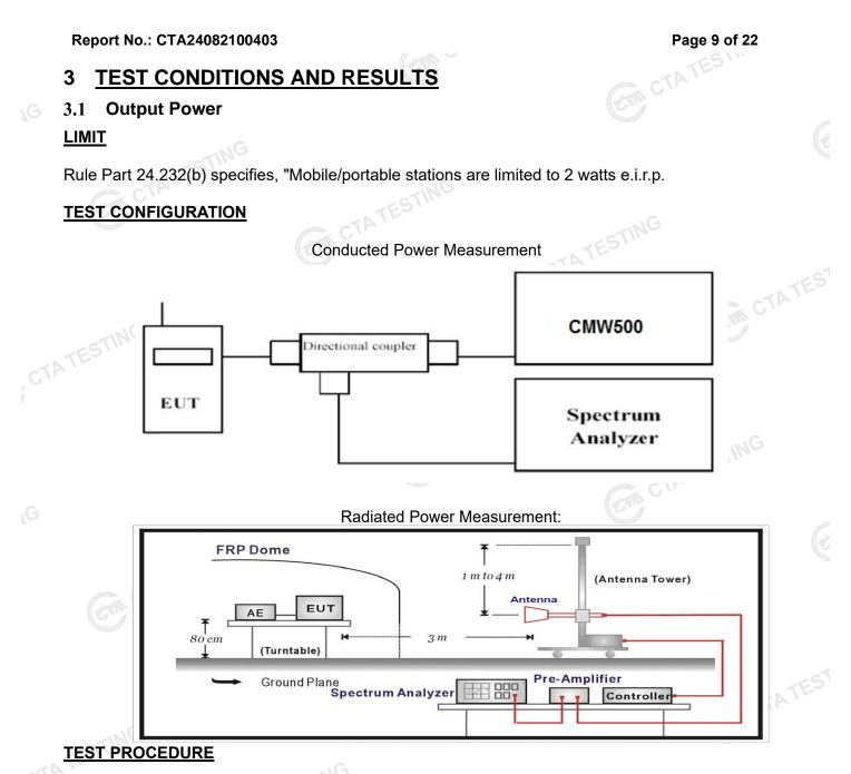
The EUT was setup according to EIA/TIA 603D
