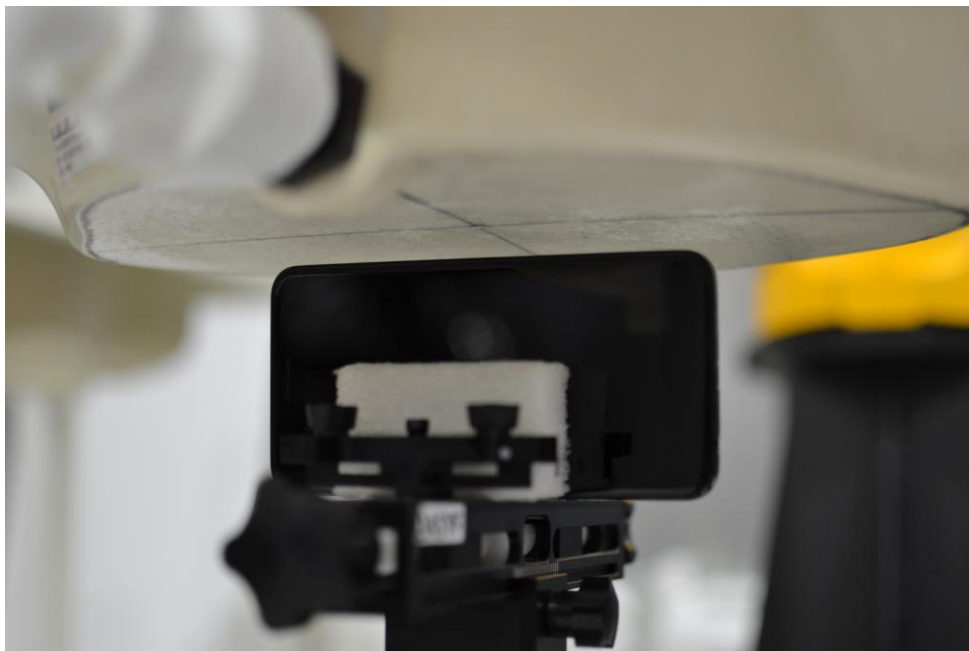
SAR Test Setup Photo 9: Right at 1.0 cm
