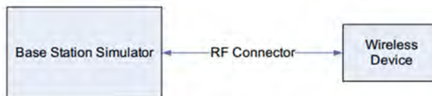
Figure 9.1 Power Measurement Setup
