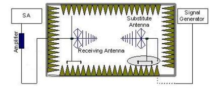
In the chamber, an substitution antenna for the frequency band of interest is placed at the
