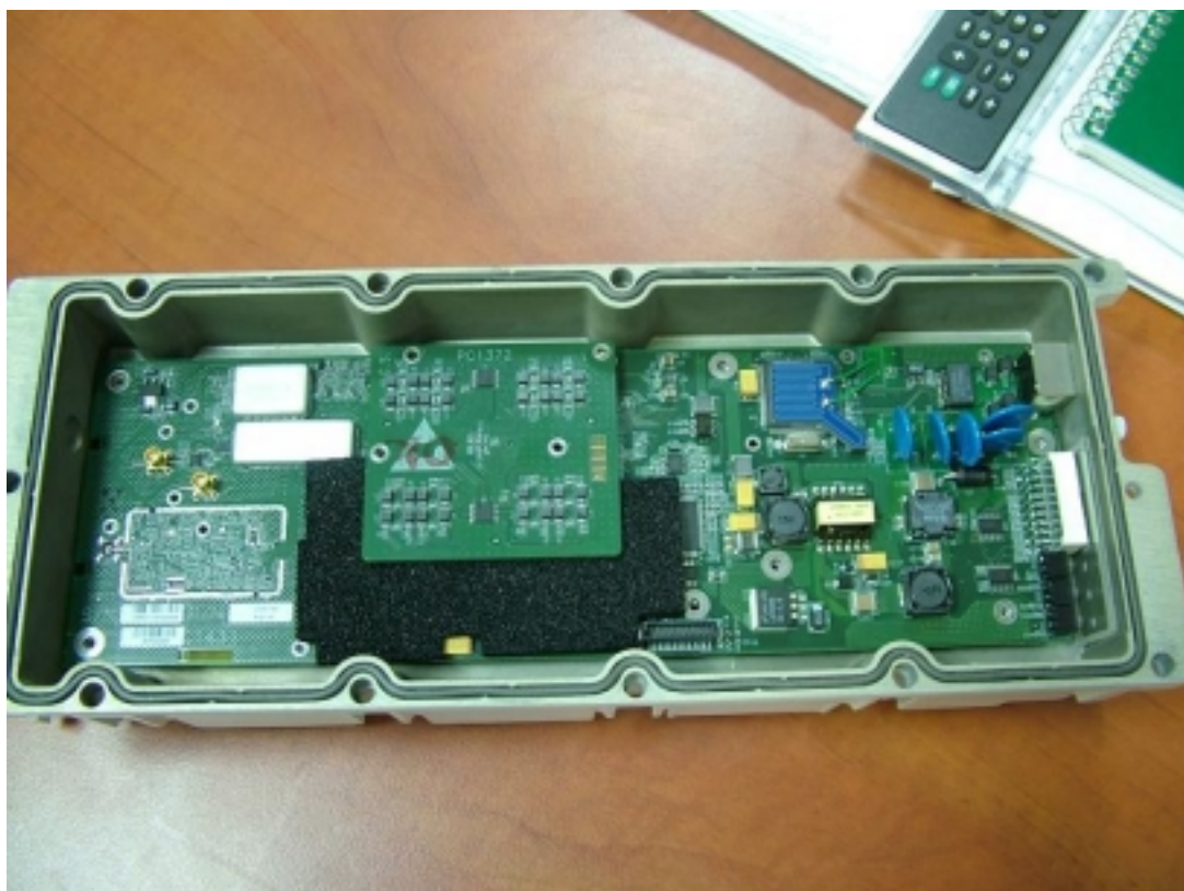
Photo # 1. Radio Unit. PWB component side
