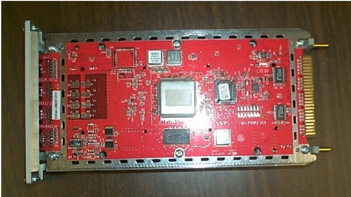
Figure 9.12: Picocell System Inside Back View of Controller Module
